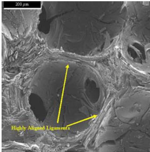
Figure 1. SEM image of graphite foam showing highly aligned graphitic ligaments.
