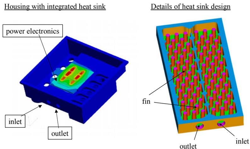
Figure 2. Housing with integrated heat sink for cooling of power electronics
