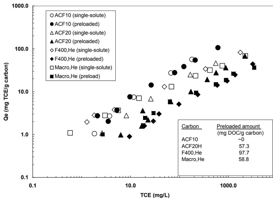
**Figure 1. TCE adsorption isotherms of various “fresh” and “preloaded” activated carbons.**
