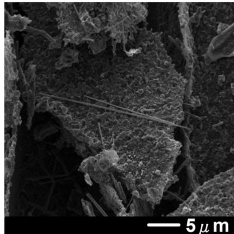
Figure 2. SEM image of the inside of a pore with SiC nanorods hanging above the one micron thick SiC coating of a pore wall in wood charcoal.
