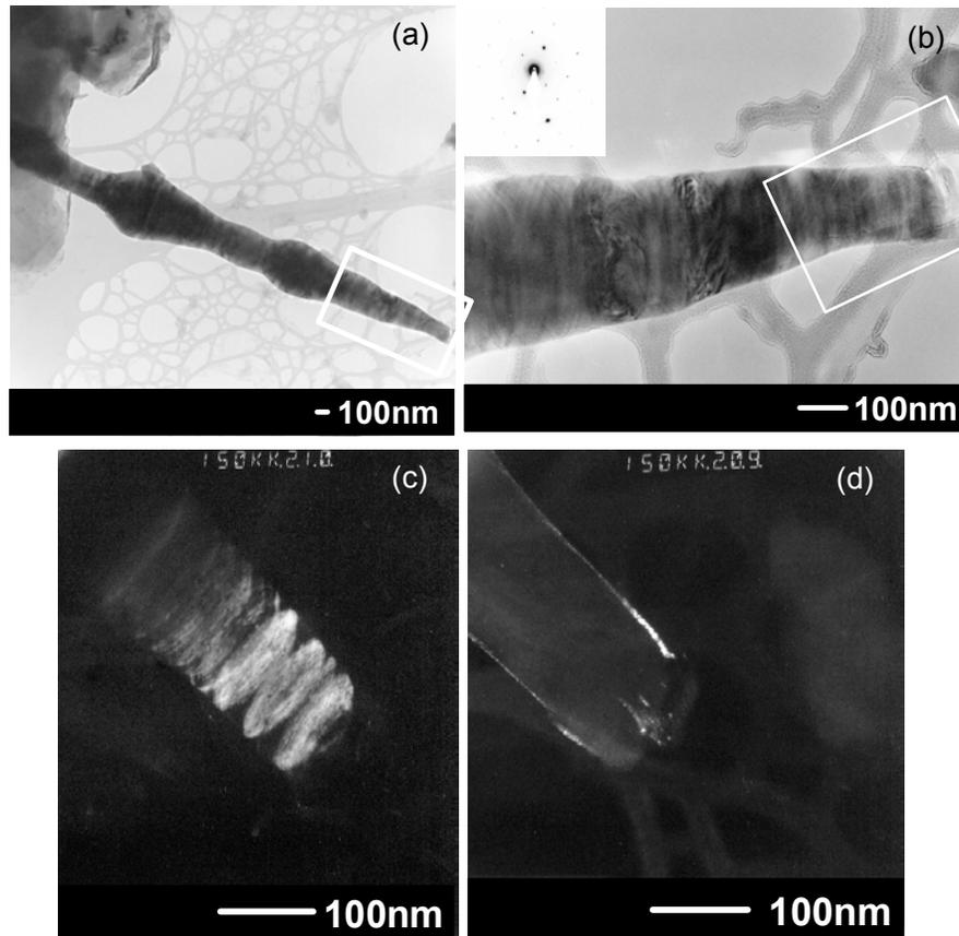
Figure 3. SiC nanorods formed together with silicon carbide coatings on pore walls in wood charcoal. (a) TEM image of bamboo like SiC nanorod. (b) TEM image of white box in (a) with SiC tip nucleus in insert is the diffraction pattern. (c) TEM dark field image of white box in (b) showing the (111) preferred growth direction. (d) TEM 002 dark field image of white box in (b) showing the graphitic carbon layer.
