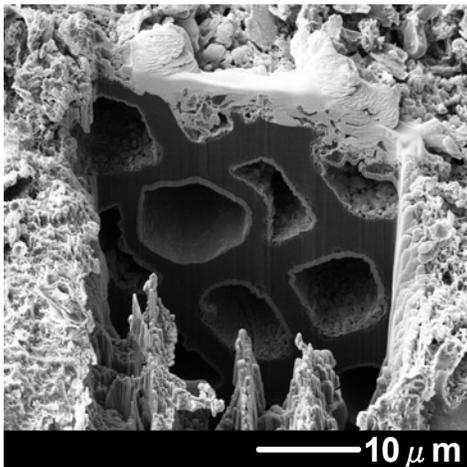
Figure 1. SEM image of FIB machined cross section of wood charcoal showing the pore walls with one micron thick SiC coating.
