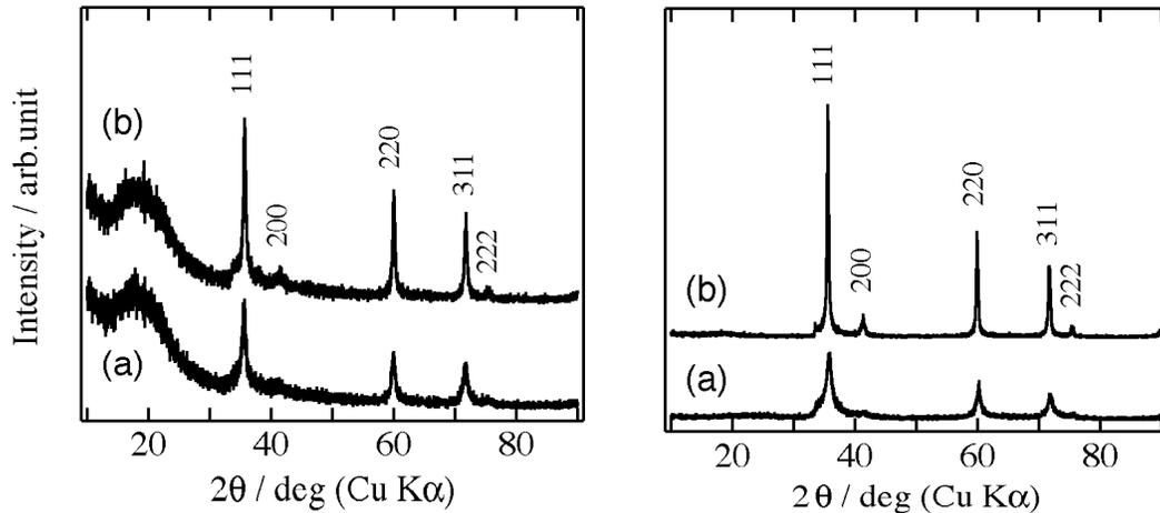
Figure 5. XRD patterns of the products from the precursor (UF No.14) by heat treatment at 1600°C for (a) 1 h and (b) 5 h in A. The left figure is for as formed blocks and the right after crushing.
