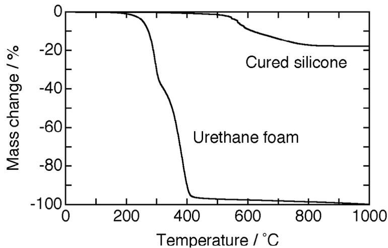
Figure 2. Thermal decomposition behavior of urethane foam and cured silicone measured at 400 K h<sup>-1</sup> in Ar.
