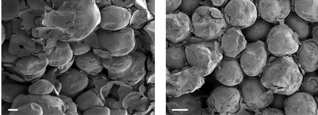
Figure 3. SEM images of 1600°C, 1 h products from precursor (UF No.14) (left) and precursor (UF HP70) (right). Bars are 100  $\mu\text{m}$ .
