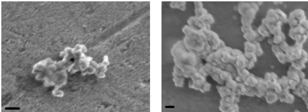
Figure 4. SEM images of 1600°C, 5 h products from precursor (UF No.14) (left) and precursor (UF HP70) (right) after crushing. Bars are 200 nm.
