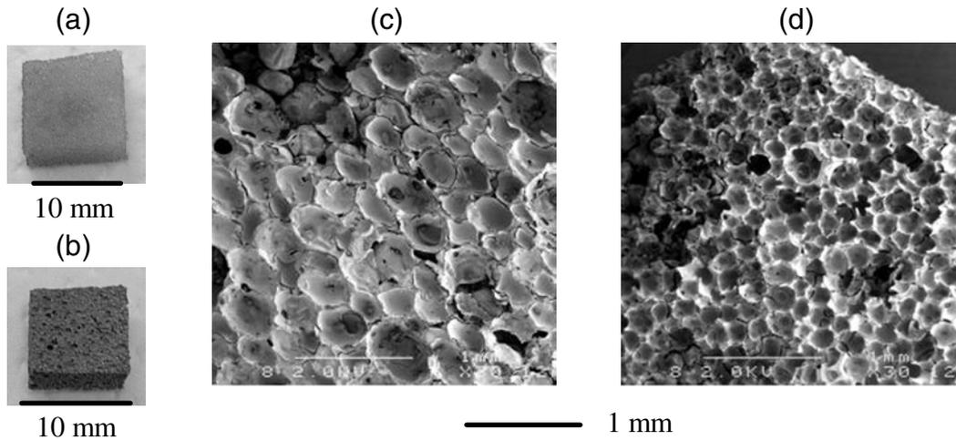
Figure 1. Photographs of (a) precursor (UF No.14) and (b) after heat treatment. SEM images of the surface of  $\beta$ -SiC formed from (c) precursor (UF No. 14) and (d) precursor (UF HP70). All were heat-treated at 1600°C for 5 h in Ar, except (a).
