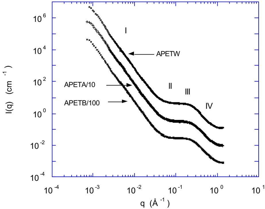
Figure 2 SAXS spectrum of the three samples APETW, APETA and APETB in air, showing the four zones described in the text. APETA and APETB have been shifted vertically downward by one and two decades, respectively.
