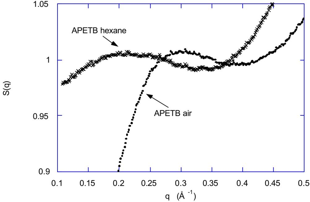
Figure 3 Structure factor  $S(q) = I(q)/P(q)$  calculated for sample APETB in air (+) and in liquid hexane (x), where  $P(q)$  is given by eq 1.
