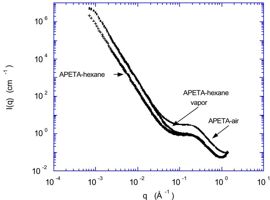
Figure 4 SAXS spectra of sample APETA in air, in hexane vapor and in liquid hexane. The APETA-hexane vapor curve is identical to that of the APETA-air sample at low  $q$ , but at  $q \geq 0.1 \text{ \AA}^{-1}$ , it joins that of the liquid hexane. This shows that hexane in the micropores is in liquid state.
