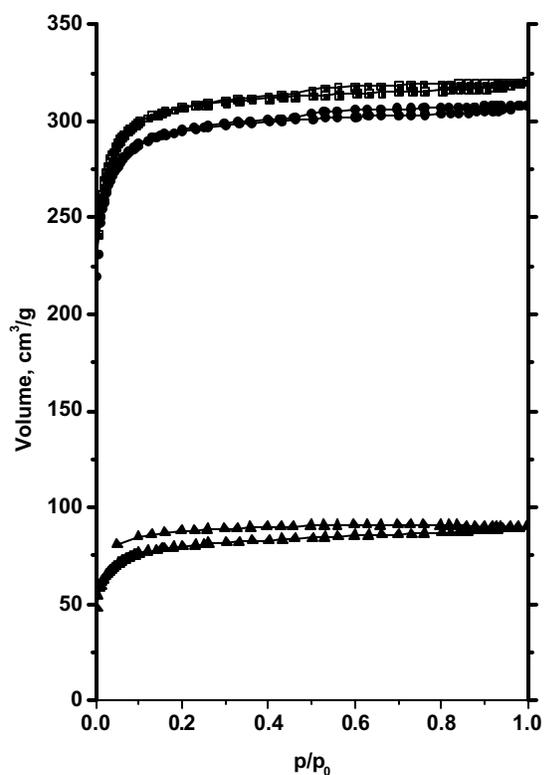
Figure 1 Low temperature nitrogen adsorption isotherms of the carbon samples. From top to bottom: APETW, APETA, APETB.
