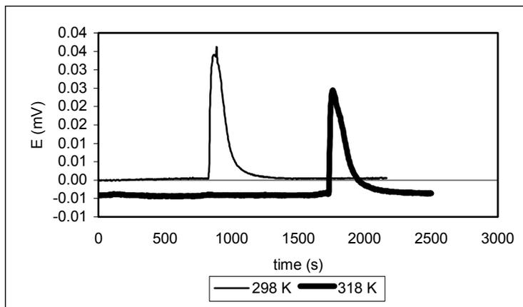
Figure 2. Thermograms obtained with the immersion of activated carbon in aqueous phenol solution at 298 and 318 K
