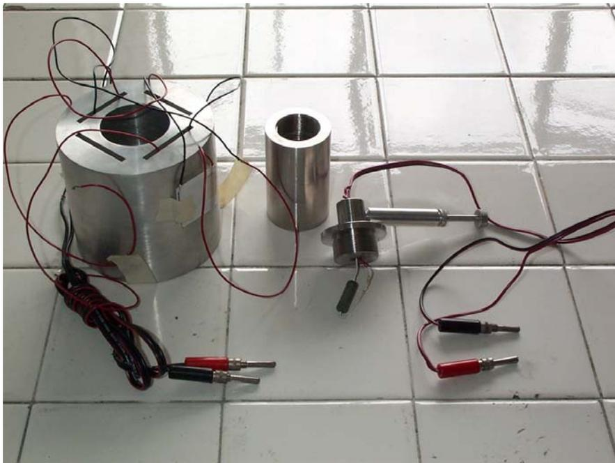
Figure 1. Heat conduction microcalorimeter with metallic cell
