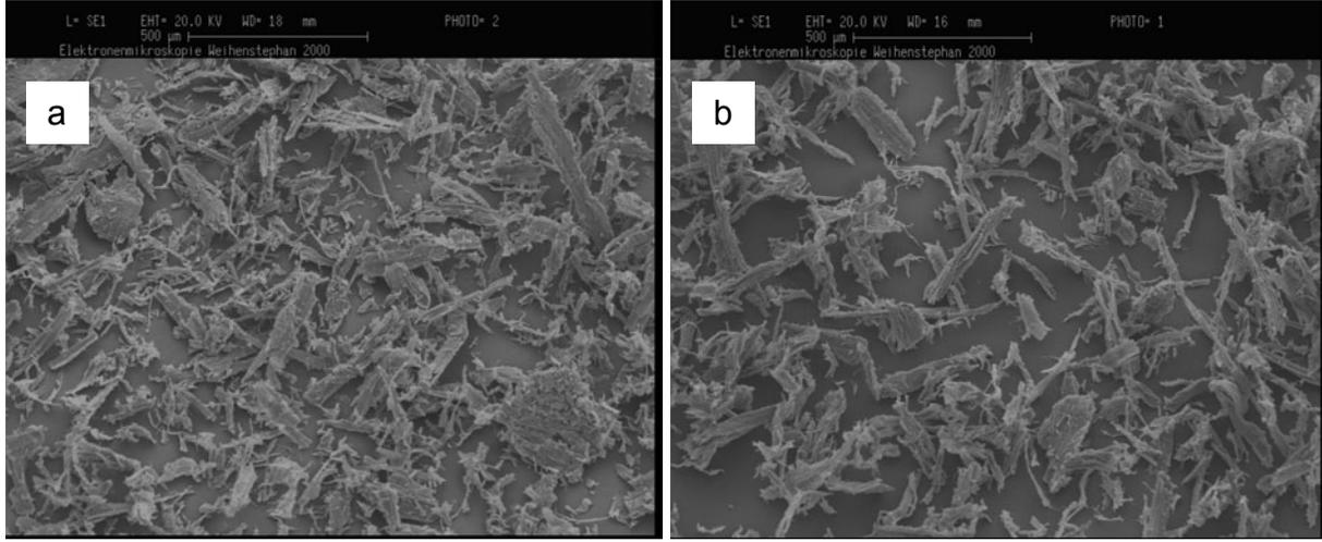
Figure 1. SEM pictures of (a) the crude and (b) the carbonised wood fibres.
