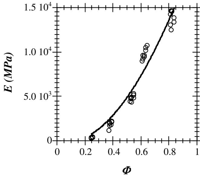
Figure 3. Elastic modulus ( $E$ ) vs the volume fraction ( $\Phi$ ) of carbon particles. The solid curve is calculated with Eq. (10).
