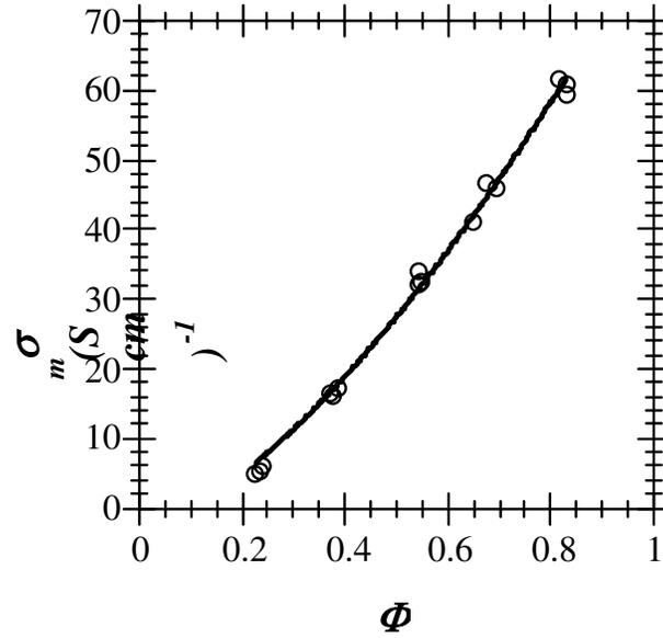
Figure 2. Electrical conductivity ( $\sigma_m$ ) vs the volume fraction ( $\Phi$ ) of carbon particles. The solid curve is calculated with Eq. (3).
