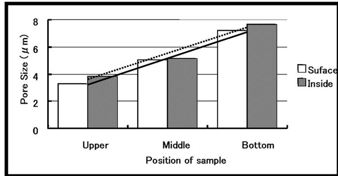
Fig.3 Pore change of this carbon
