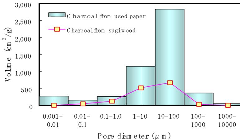
Fig.1 Pore distribution of carbon made from woody materials and traditional carbon
