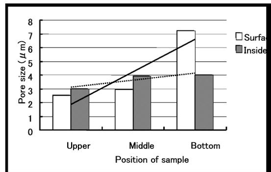
Fig.2 Pore change of this carbon
