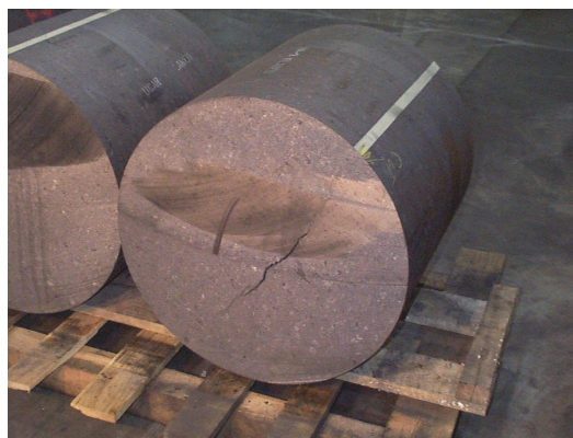
Figure 2. Typical Ultrasonic Discovered Artifact
