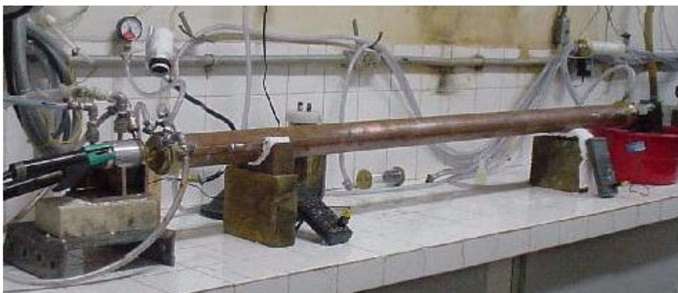
Fig. 2. The plasma torch at left, connected at a tubular reactor.
