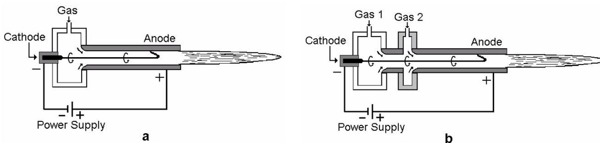
Fig. 1. Plasma torch: a) with one vortex chamber ; b) with two vortex chambers.
