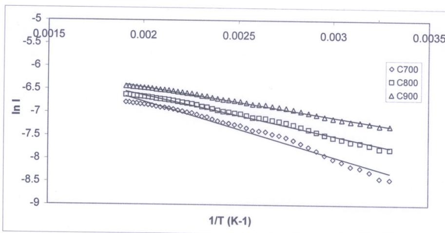
Fig. 1. Temperature dependence conductivity of different carbons measured from 30 to 250 C
