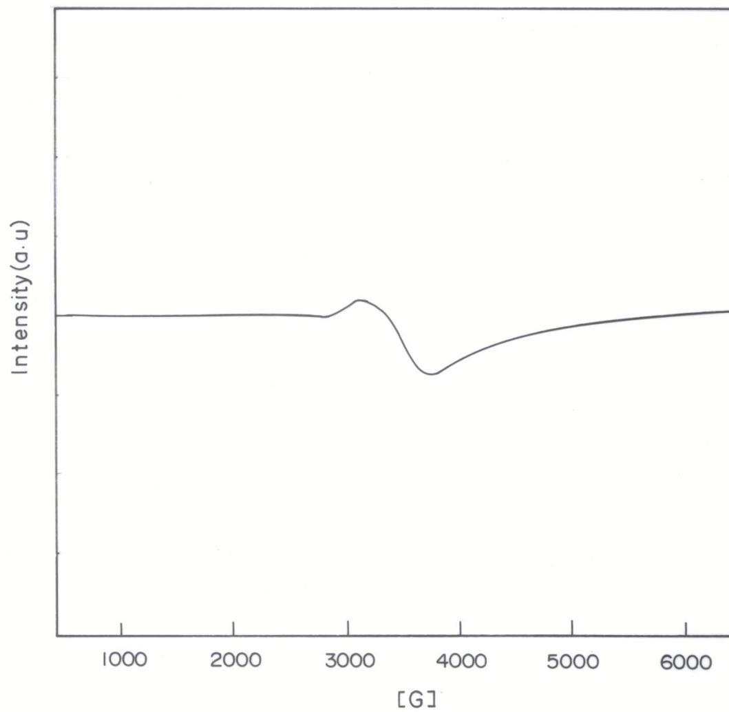
Fig. 6. Electron spin resonance spectra of C900 carbon sample.
