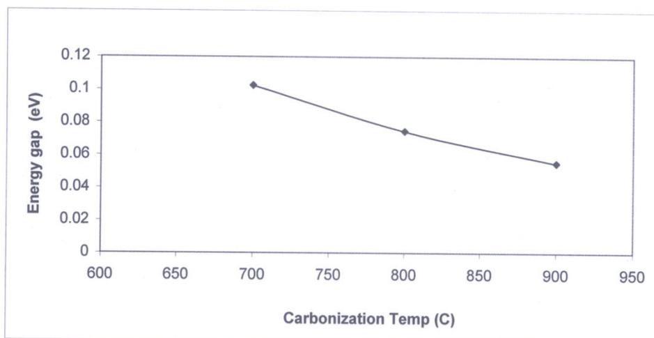
Fig. 2. Estimated energy gap for hopping conduction in carbon powders at different carbonization temperature
