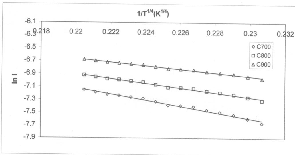
Fig. 3. Temperature dependence conductivity of different carbons measured from 80 to 150 C
