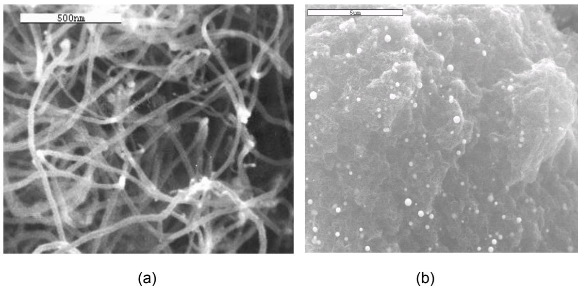
Figure 1. SEM images of (a) CNTs alone; (b) CNTs with Pt-Ru particles
