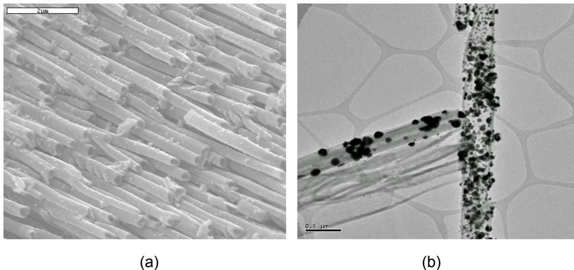
Figure 2. (a) SEM (b) TEM image of template CNTs with electrodeposited Pt-Ru particles
