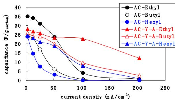
Fig.2 Capacitances of mesoporous (AC-Y-A) and microporous (AC) carbons in R<sub>4</sub>NBF<sub>4</sub>/propylenecarbonate(PC) solutions
