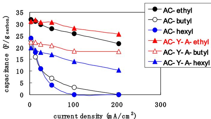
Fig.3 Capacitances of mesoporous (AC-Y-A) and microporous (AC) carbons in R<sub>4</sub>NBF<sub>4</sub>/acetonitrile(AN) solutions
