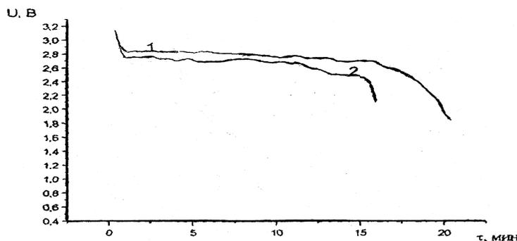
Fig. 1. Discharge characteristics of nickel-carbon cathode
