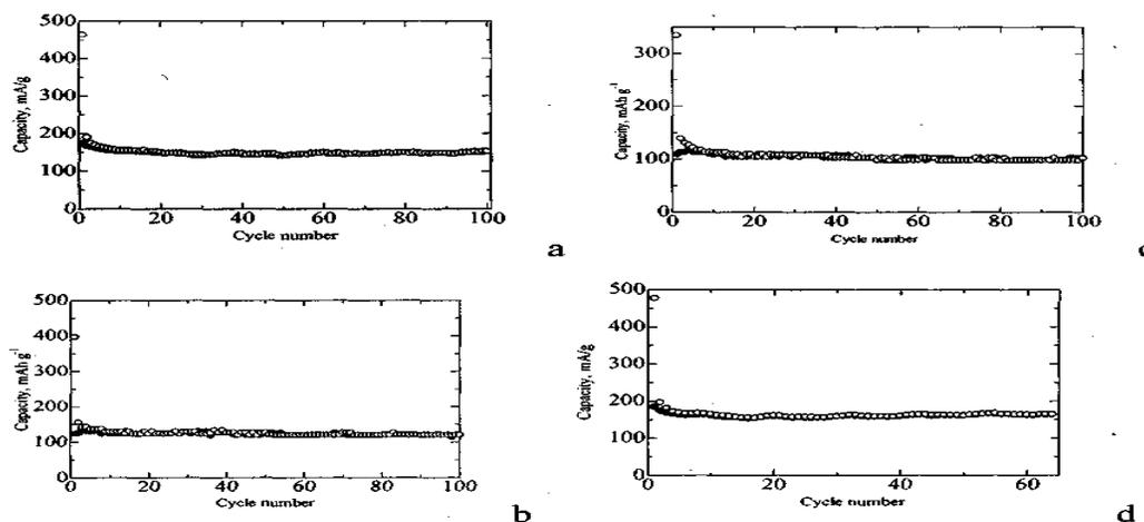
Fig. 2. Cycling performances of Li/1 mol l-1 LiClO<sub>4</sub> in EC:DEC=1:1/ABR
