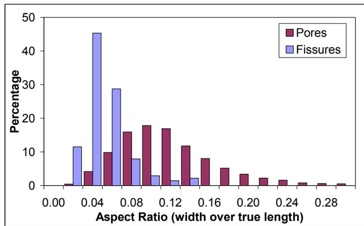
Figure 3 Aspect Ratio for Fissures and Pores
