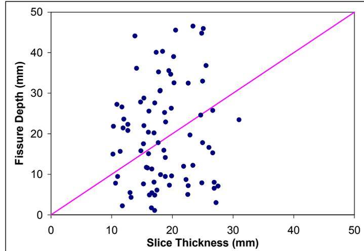
Figure 5 Coke Slice Cross-Sections perpendicular to the observed Fissures: Fissure depth relative to the Slice Thickness
