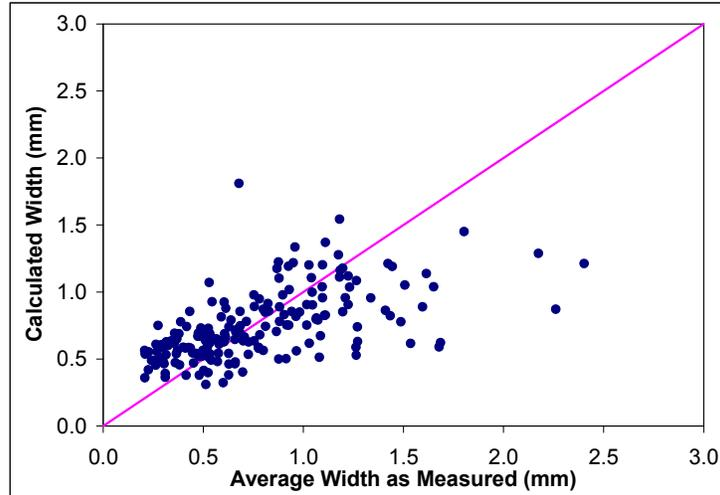
Figure 4 Comparing the Average Measured and the Calculated Fissure Width
