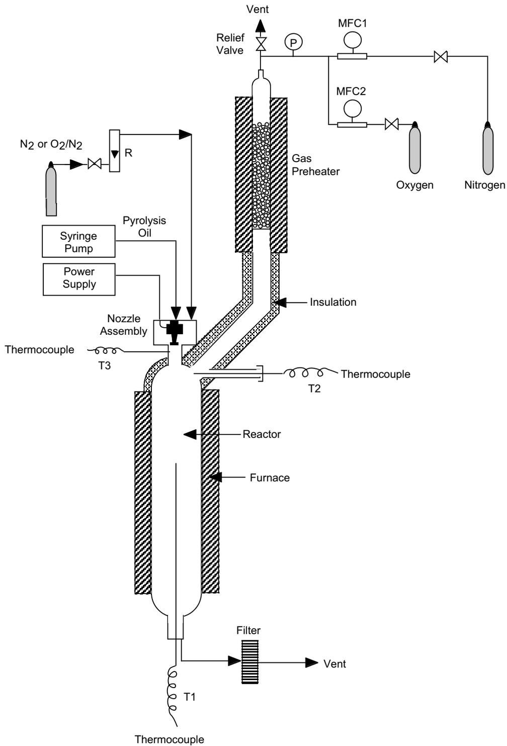
Figure 1. Experimental set-up used to produce carbon black. *MFC1* and *MFC2* are mass-flow controllers, *T1*, *T2*, and *T3* are thermocouples, *R* is a rotameter and *P* is a pressure gauge.
