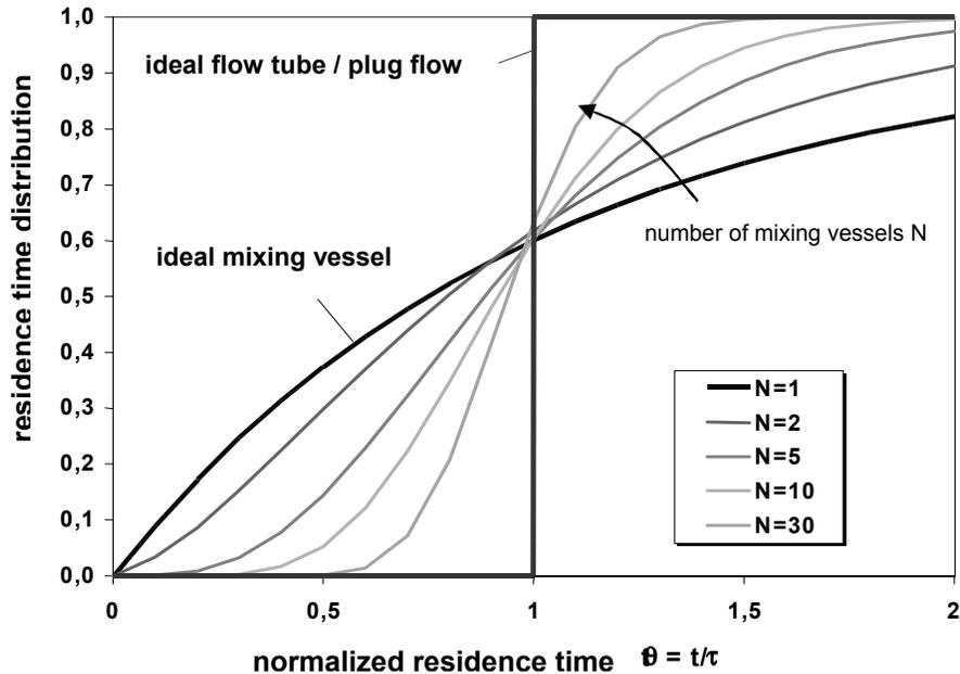
Figure 5. Residence time distribution sum according to the cascade model
