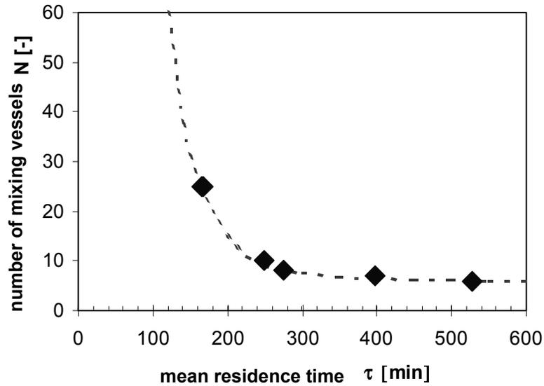
Figure 6. Model parameter “Number N of mixing vessels” depending on the mean residence time  $\tau$  of carbon black in the bead drum
