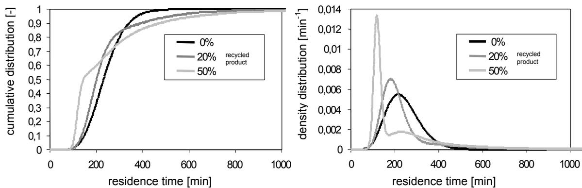
Figure 7. Change of residence time distribution depending on the quantity of recycled product
