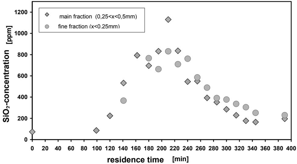
Figure 2. Measured SiO<sub>2</sub> concentration at the drum exit, as a function of test duration
