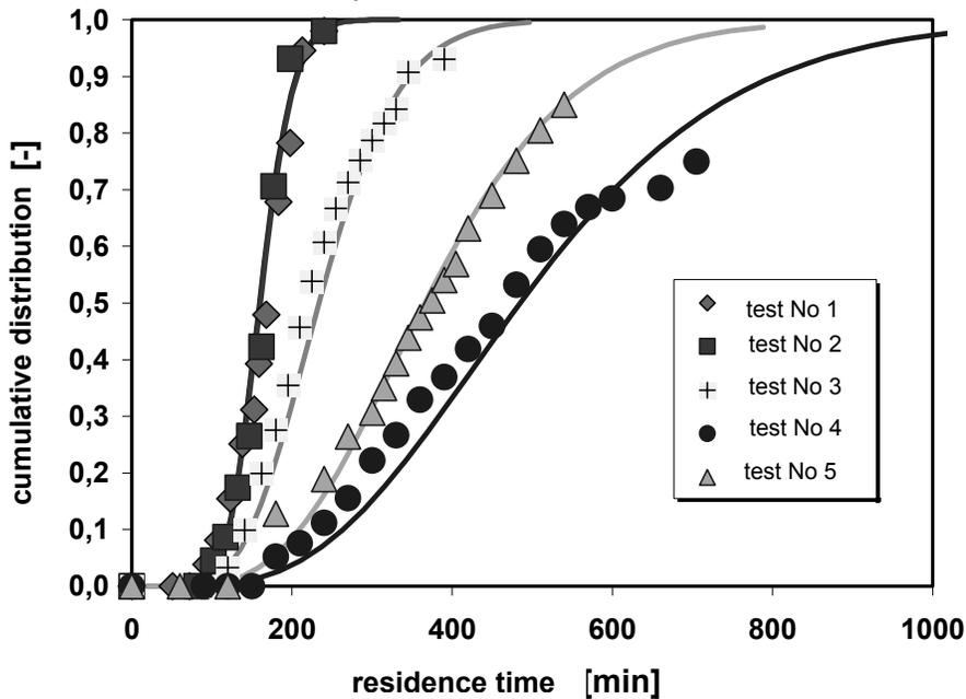
Figure 3. Measured and calculated residence time distribution sums (cf. Sections 3 and 4)
