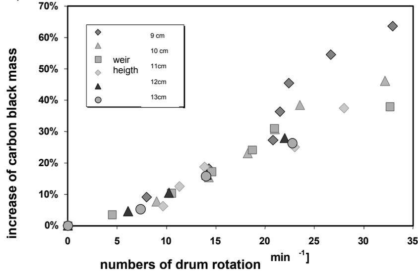
Figure 4. Increase of carbon black bed mass in rotating drum (D = 0.52 m)
