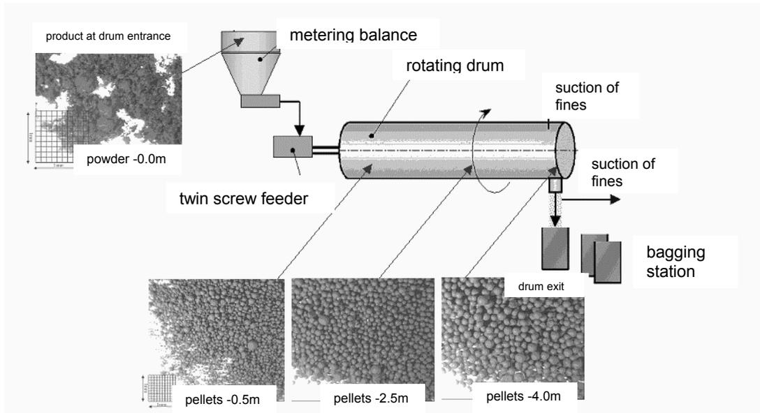
Figure 1. Schematic view of the experimental setup – bead-forming drum with metering balance, twin screw conveyor and various granulation stages
