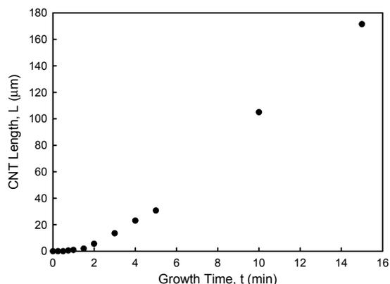
Fig. 4. CNT length as a function of time.
