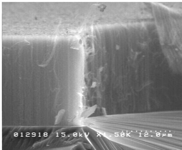
Fig. 3. An SEM image showing cross-sectional view of high-density aligned carbon nanotubes grown on Fe-Si.
