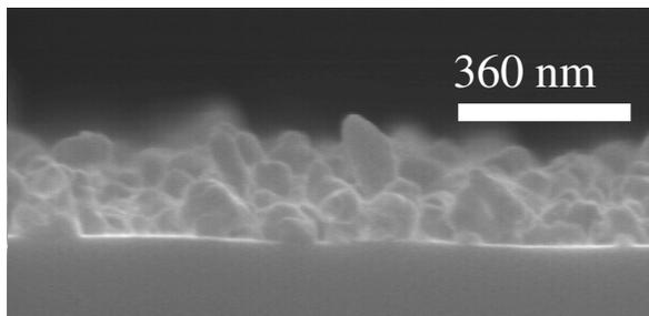
Fig. 2. SEM image shows that carbonaceous clusters were synthesized using pure Fe film as a catalyst under 500 W, CH<sub>4</sub>/H<sub>2</sub> = 2/9 and 25 Torr for 3 min.
