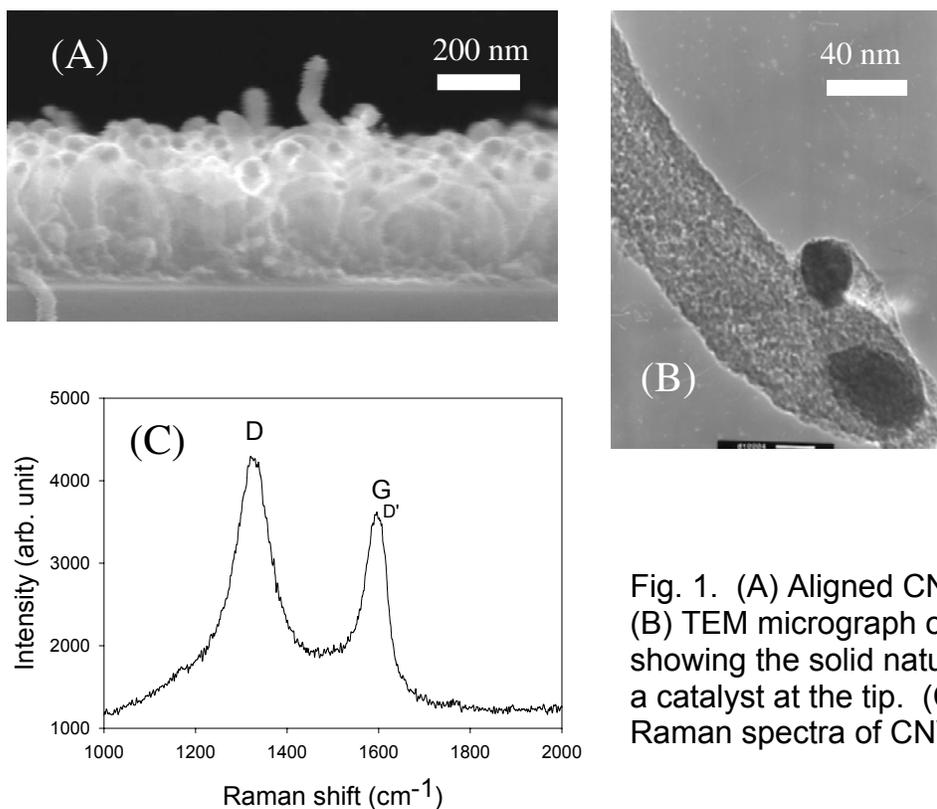
Fig. 1. (A) Aligned CNWs. (B) TEM micrograph of CNW showing the solid nature and a catalyst at the tip. (C) Raman spectra of CNW.
