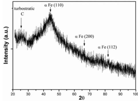
Figure 1. X-ray diffraction spectra of Fe-C nanocomposite powder.
