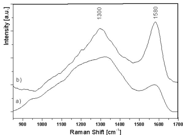
Figure 7. Comparison between the Raman spectra of Fe/C nanocomposites (sample F - curve a) and a nanocarbon sample issued by laser pyrolysing the same hydrocarbon precursors.
