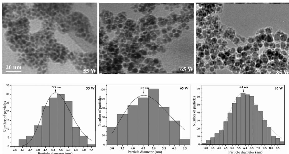
Figure 4. TEM images and corresponding particle size distributions for Fe/C samples obtained at increasing laser radiation intensity: 55 W (sample C), 65 W (sample B) and 85 W (sample A)
