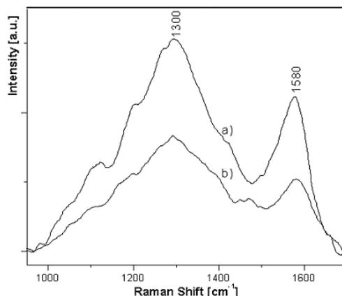
Figure 6. Raman spectra for two different Fe-C nanocomposite samples, obtained at two different reactor total pressures: a-sample D (650 mbar) and b-sample E (450 mbar)
