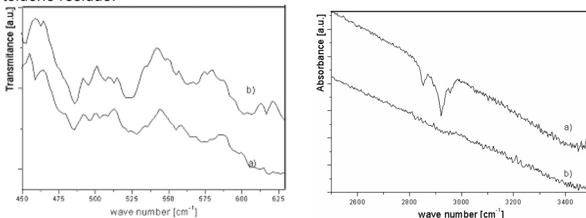
Figure 8. FTIR spectra of F Fe/C nanocomposite sample (a) and its residue (b) in the  $400\text{-}700\text{ cm}^{-1}$  (left side) and  $2000\text{-}3500\text{ cm}^{-1}$  (right side) wave-number regions. Spectrum (b) has been obtained from the dried residue of the toluene extract, i.e. from the nonsoluble part collected in the filter.
