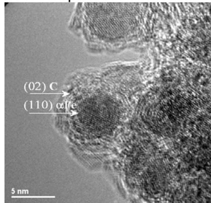
Figure 2. HRTEM images showing typical shell core structures of Fe/C nanoparticles (sample A)
