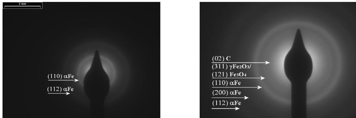
Figure 5. SAED patterns for Fe/C nanoparticles, sample A (on the left side) and sample B (on the right side).
