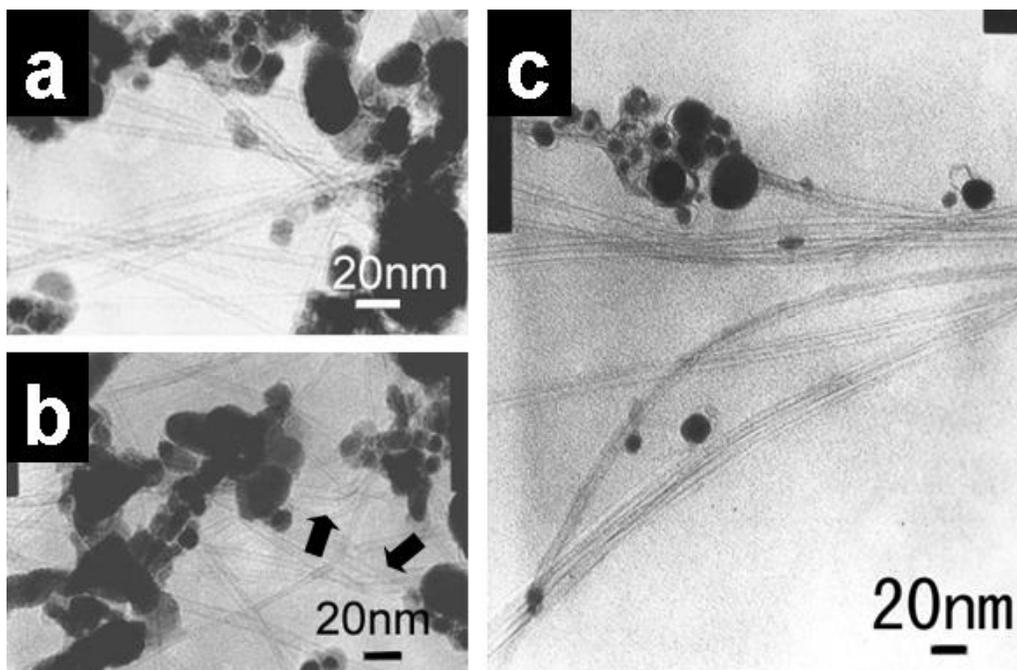
Fig. 2. TEM images of nanotubes with thin walls; (a) An image showing many thin-walled nanotubes with a big diameter exist in discrete state; (b) Some thin-walled nanotubes with distorted sections, as pointed by black arrows; (c) Nanotubes with thin walls, which was prepared from coal-derived carbon rods obtained at 1173 K.
