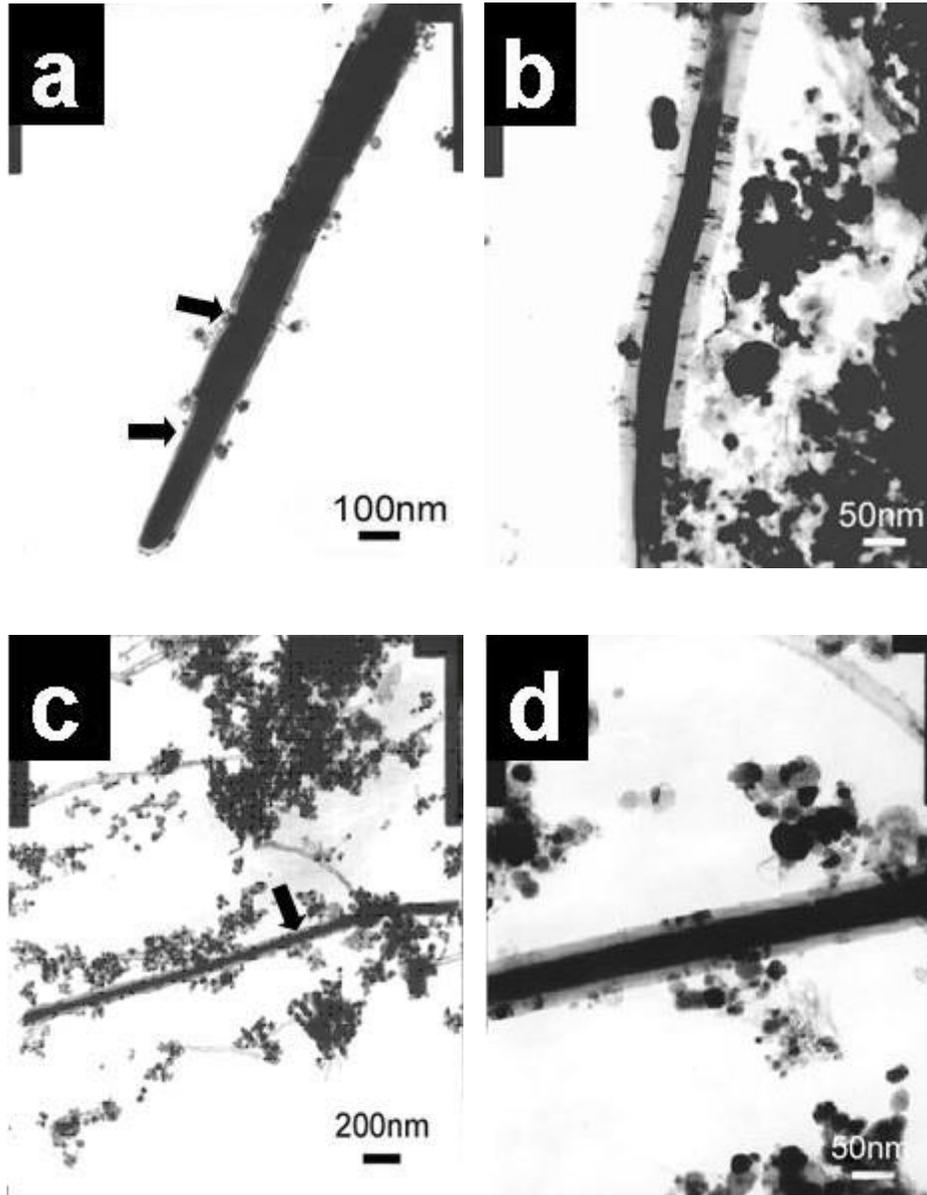
Fig. 1 TEM images of CNTs completely filled with metal-based materials. (a) One CNT of about 1.5  $\mu\text{m}$  in length that is filled with continuous Cr species, in which sudden changes in the tube diameter are marked by arrows; (b) A CNT filled with Fe species; (c) A typical image of Ni-species filled CNT or nanowire with a uniform diameter and a length over 2.6  $\mu\text{m}$ ; (d) A high magnification image of the arrow-marked section of the Ni-filled CNT shown in Fig. 1c.
