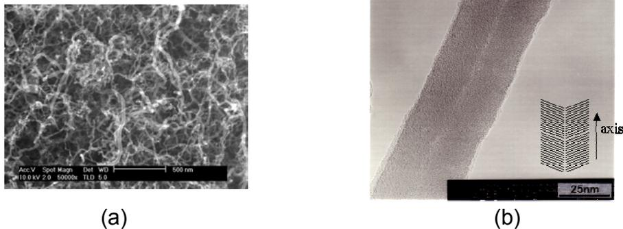
Fig. 1. SEM and TEM image of herring-bone types carbon nano fibers.
