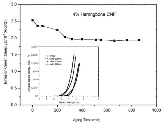
Fig. 4. The electrical aging and degradation of carbon nano fiber emitters.
