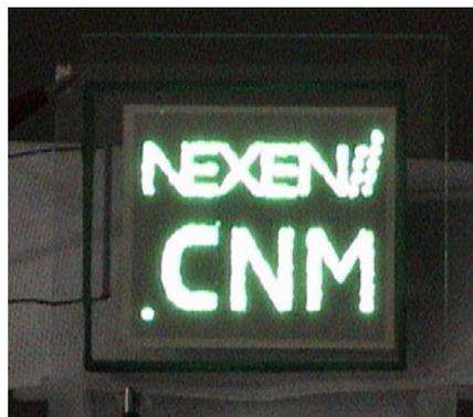
Fig. 5. The field emission image of HB-CNF emitters with fully vacuum packaged panel.
