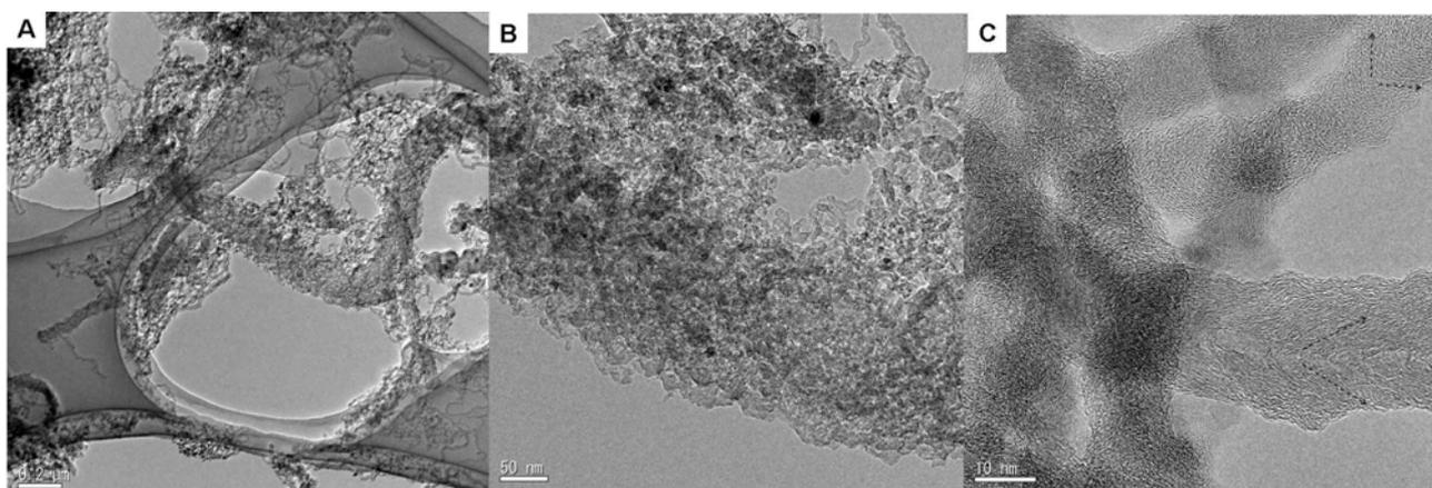
Figure 2. TEM images of CNF over 5% Ni supported on CB at 480°C.
