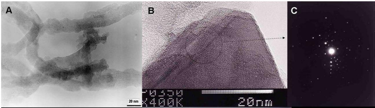
Figure 4. TEM images of CNF and catalyst particle, and the electron diffraction of the catalyst particle after synthesis using 5% Ni-Fe (8:2) supported on CB at 480°C.
