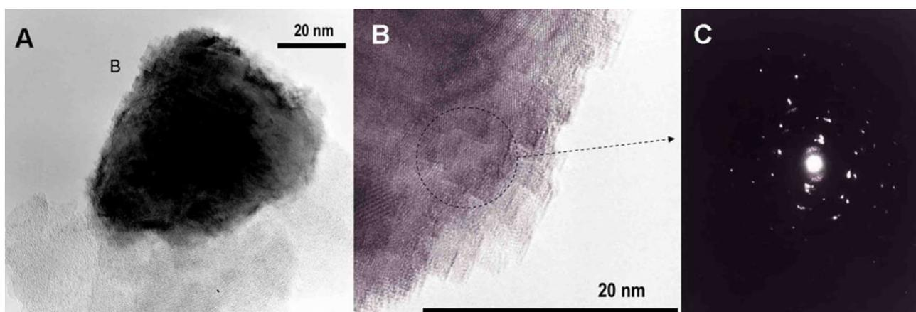
Figure 3. TEM images and electron diffraction at a selected area of Ni alone supported on CB after synthesis of CNF at 480°C.
