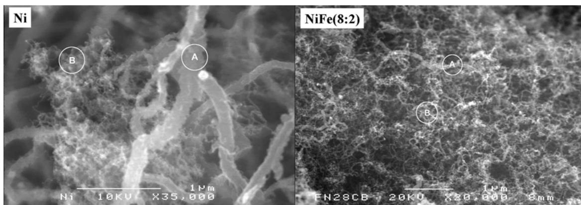
Figure 1. SEM images of CNFs from  $C_2H_4/H_2$  (4:1) at 753 K on the 5% Ni alone and 5% Ni-Fe (8:2) supported on MCB#3050B
