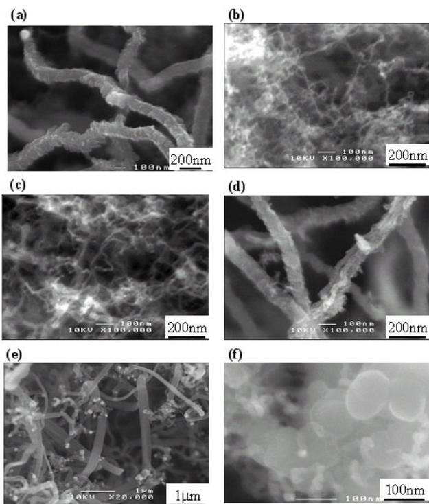
Figure 2. SEM images of products from ethylene/H<sub>2</sub> (4:1) at 480°C for 1 h using CB-supported Fe-Ni, of which metal composition is: (a) Ni, (b) Ni-Fe (9:1), (c) Ni-Fe (8:2), (d) Ni-Fe (7:3), (e) Ni-Fe (6:4), and (f) Ni-Fe (5:5).
