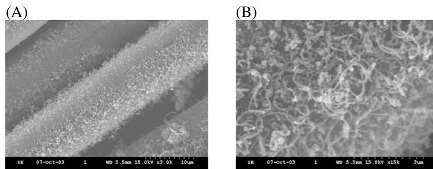
Figure 1. SEM images of (A) CNTs grown on activated carbon fibers at 800°C and (B) their high magnitude
