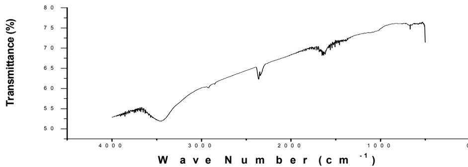
Figure 3. FTIR spectrum of fabricated CNTs that were washed by nitric acid
