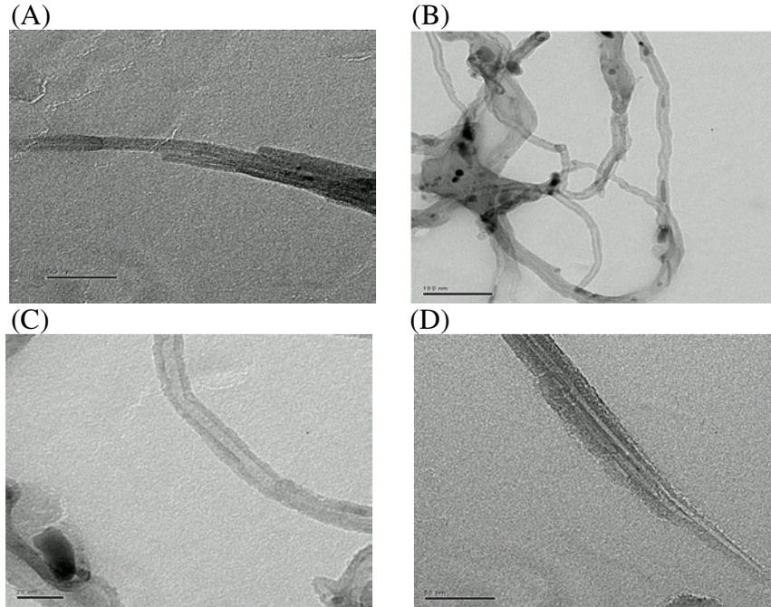
Figure 2. HR-TEM images of the grown CNTs on the activated carbon fiber surface
