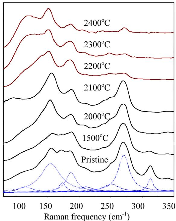
Figure 1. Low frequency Raman spectra of DWNTs (grown by a catalytic CVD method at around 875°C) heat treated at various temperatures from 1500 to 2400°C. The tendency to downshift the RBM frequency with increasing heat treatment temperature indicates the formation of thermally stable large-diameter tubes.
