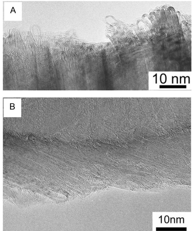
Fig. 1 HRTEM micrographs of carbon nanofiber (A) and nanotube (B) after heat-treatment at 2500°C.
