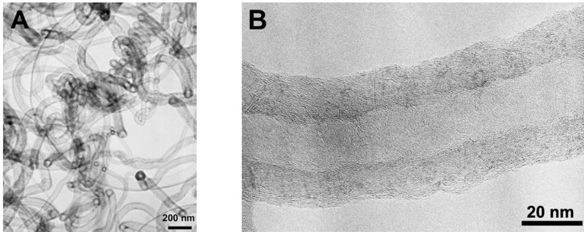
Fig. 1 Carbon nanotubes synthesized using  $\text{Co}_{0.7}\text{Fe}_{0.3}$  as catalyst at 700°C.
