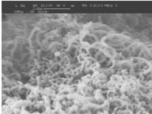
Fig 1. SEM micrograph of CNTs grown on Co-Mo/MCM-41 at 700°C
