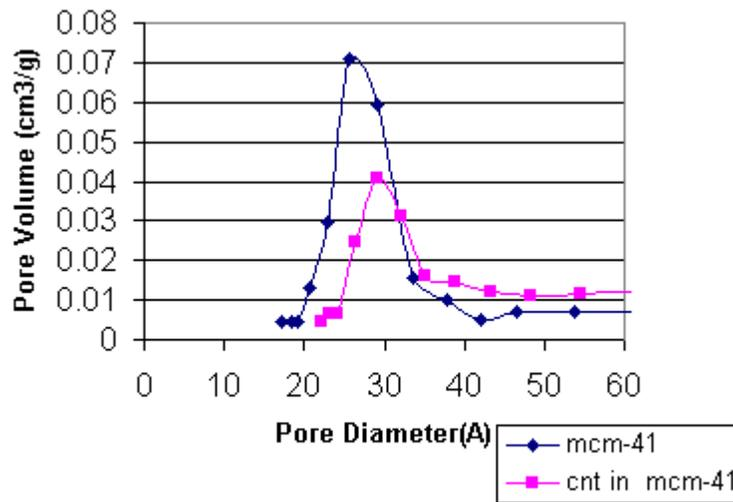
Fig 5. Pore size distribution curves for (a) MCM-41 (b) CNT in MCM-41
