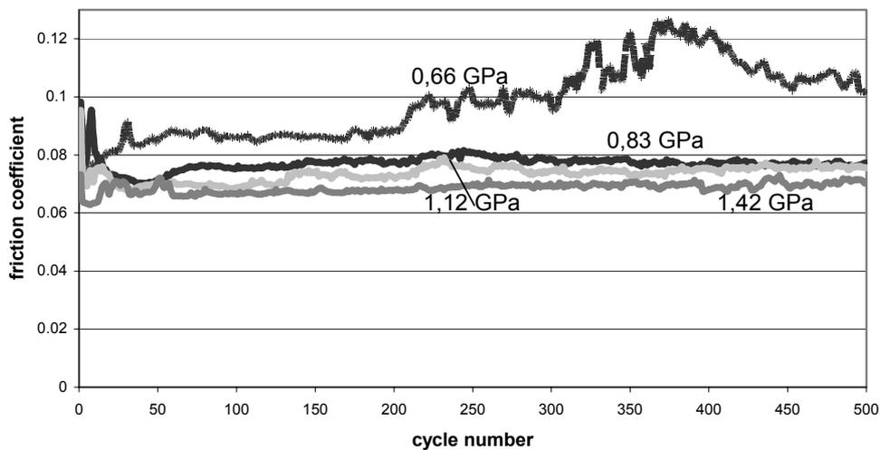
Figure 5: Evolution of friction coefficient for 1wt% SWNTs in PAO - Influence of contact pressure
