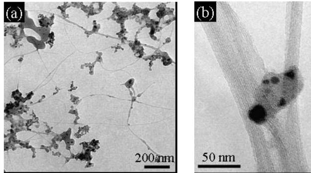
Figure 2: TEM images of SWNTs synthesised by electric arc discharge
