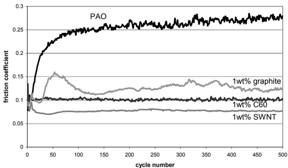
Figure 4: Comparison of different carbon forms added at 1wt% to PAO
