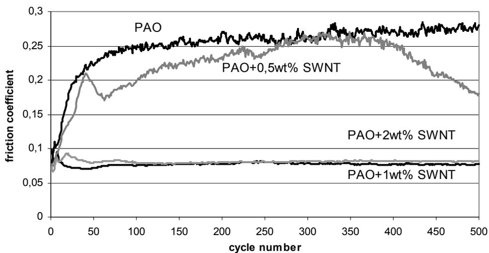
Figure 3: Evolution of friction coefficient in a lubricated contact: influence of nanotubes concentration in PAO
