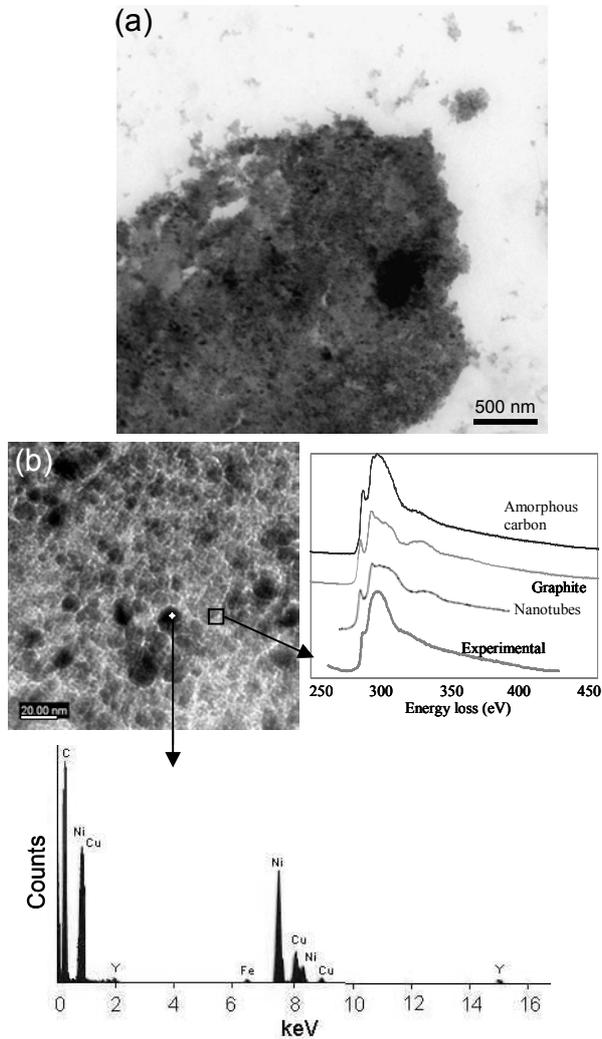
Figure 6 : TEM image of carpet-like wear debris collected from the pin: a) low magnification, b) higher magnification with corresponding EELS and X-Ray analysis performed in the black frame and on the arrowed particle, respectively
