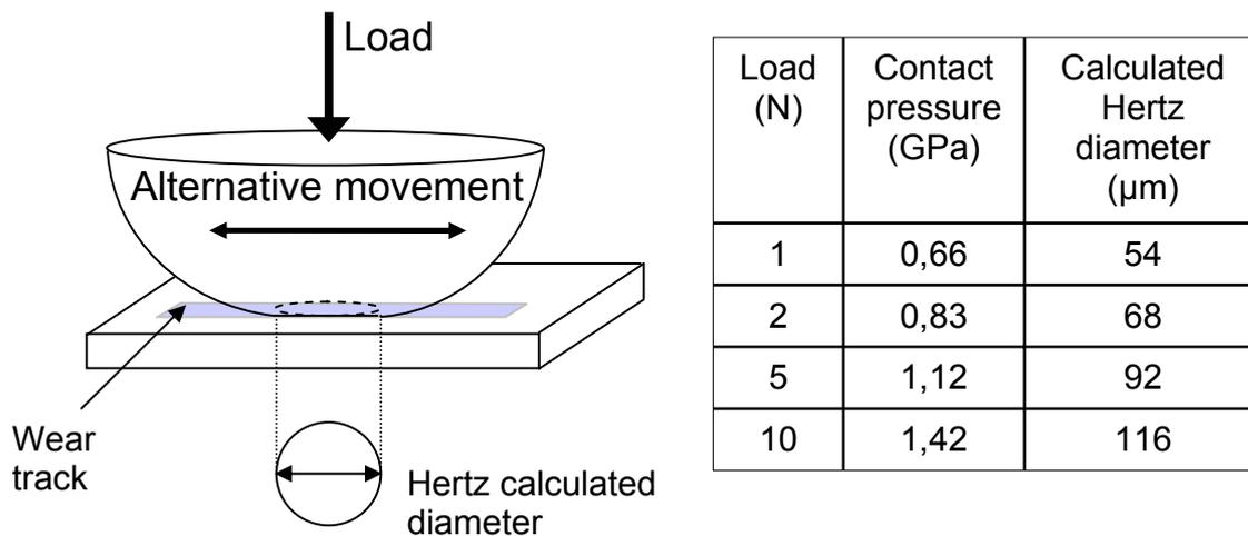
Figure1 : Pin-on-flat tribometer principle
