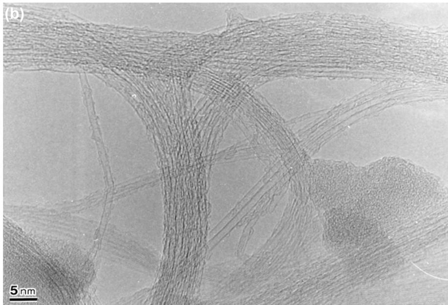
Figure 1. TEM images of (a) MWNTs and (b) SWNTs grown at 650°C and 900°C, respectively, using zeolite support
