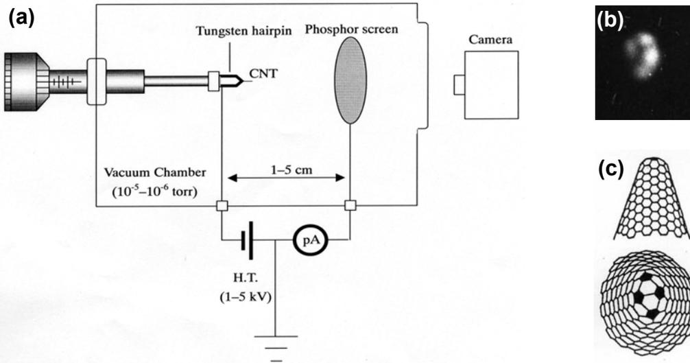
Figure 3. (a) Schematic diagram of the FEM set-up; (b) Emission pattern reflecting four-fold symmetry of an individual CNT tip; (c) Speculated structure of the corresponding CNT tip
