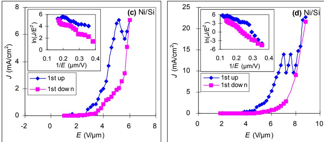
Figure 2. Field emission  $J$ - $E$  curves and corresponding F-N plots (inset) obtained from the four ANT samples
