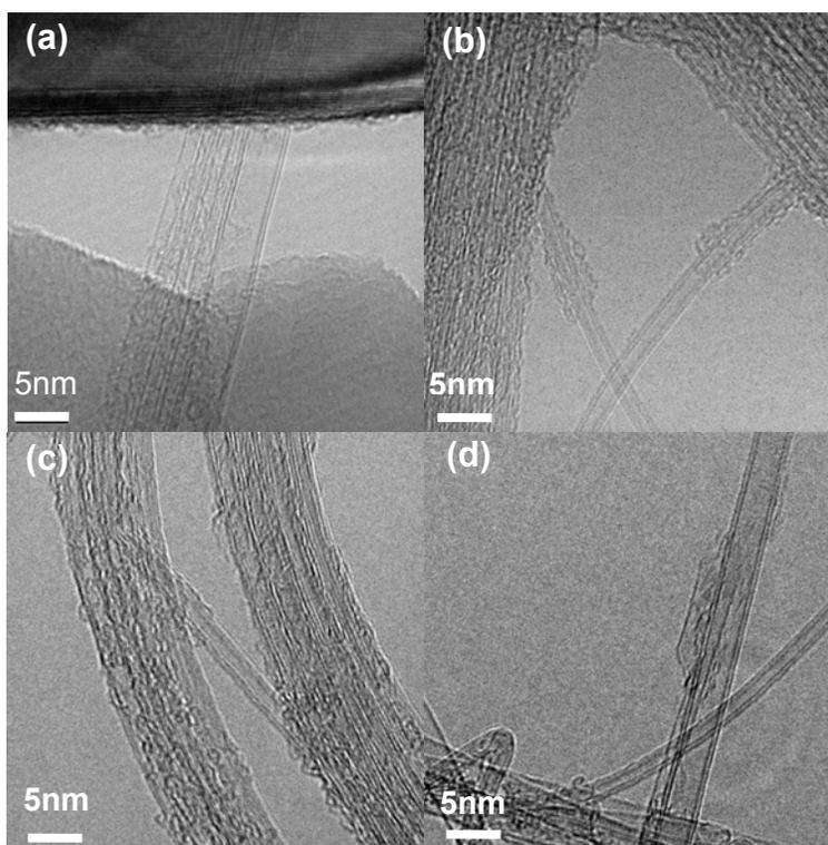
Figure 2. High resolution TEM images of DWNTs synthesized at 875°C without conditional catalyst (a), at 875°C with conditional catalyst (b), at 900°C with conditional catalyst (c) and at 950°C with conditioning catalyst.
