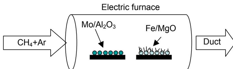
Figure 1. Schematic diagram of catalytic CVD apparatus for the synthesis of DWNTs
