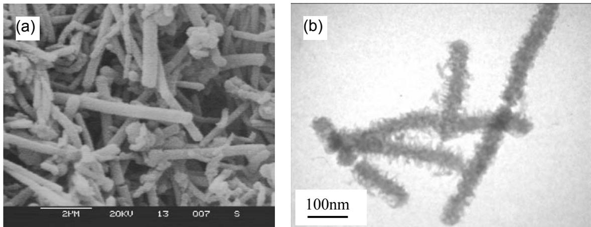
Figure 2. SEM (a) and TEM (b) images of MWNT/PANI composites
