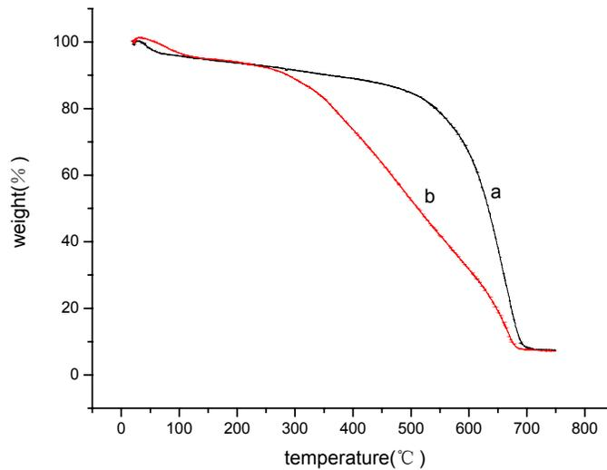
Figure 5. Thermogravimetric analysis for MWNT (a) and MWNT/PANI (b) composites
