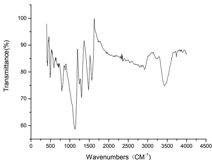
Figure 3. FT-IR spectra of MWNT/PANI composites
