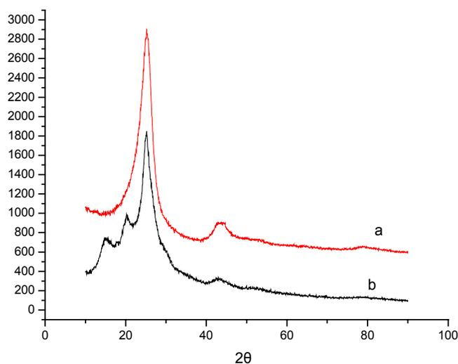
Figure 4. XRD patterns of MWNT (a) and MWNT/PANI (b) composites
