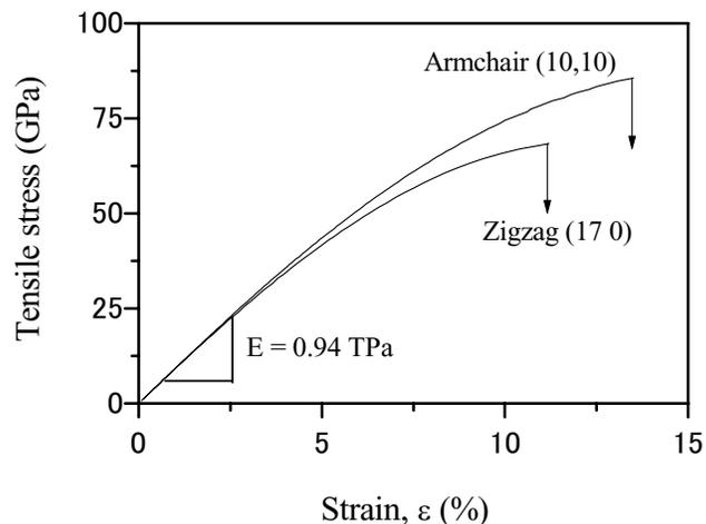
Figure 1. Stress-strain curves for the zigzag and armchair tubes under tensile load
