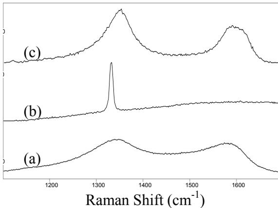
Figure 3. Typical Raman spectra of films grown on (a) untreated Si, (b) diamond-coated Si and (c) Ni-coated Si
