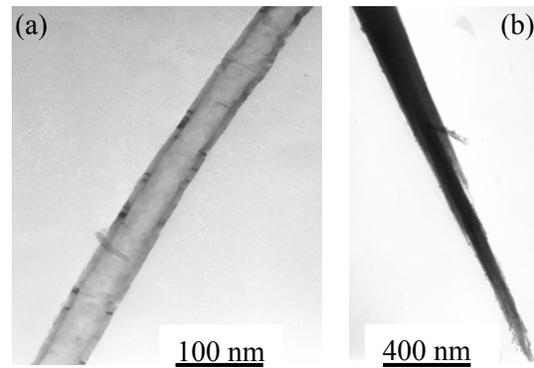
Figure 4. TEM image of typical carbon (a) nanotube and (b) nanocone
