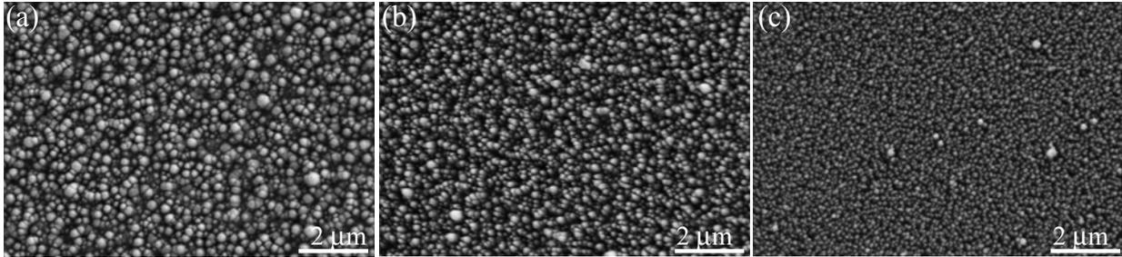
Figure 2. SEM micrographs of the films (located in the central region of the samples) grown on (a) untreated mirror polished Si, (b) CVD diamond-coated Si, and (c) Ni coated Si
