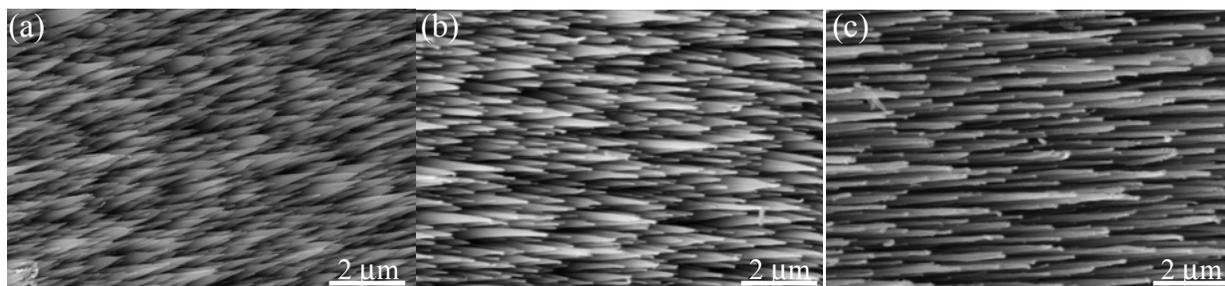
Figure 1. SEM micrographs of the films (located at the right edge of the samples) grown on (a) untreated mirror polished Si (top-right), (b) CVD diamond-coated Si and (c) Ni coated Si
