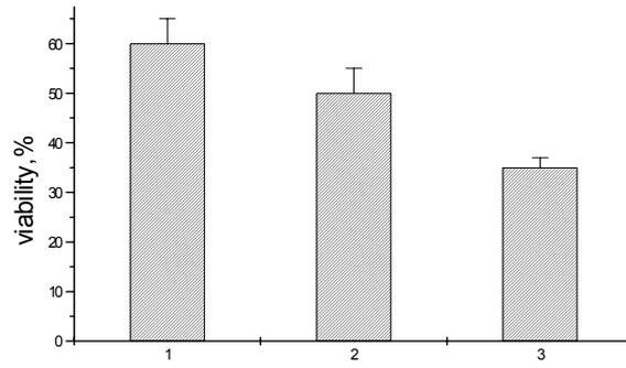
Fig. 1 Viability of fibroblast cells (human line HS5) in contact with the surface of : 1- pure polymer, 2- carbon fibers – based polymer, 3- chemically modified carbon – fibers – based composite
