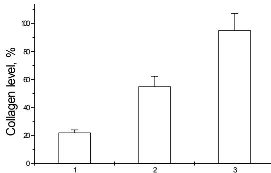
Fig.3 Collagen I level produced by osteoblasts on the surface of :1- pure polymer, 2- carbon fibers- based composite, 3- chemically modified carbon fibers – based composite
