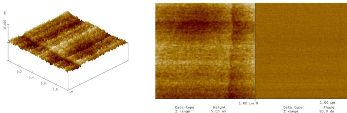
Figure 1. TM-AFM height and phase images of a plasma modified HOPG surface.
