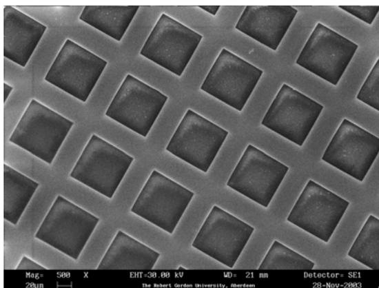
Figure 2. SEM image of a patterned graphite surface (acetone plasma treated for 10min)
