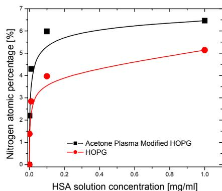
Figure 5. Nitrogen atomic percentage as measured using XPS variation function of the solution concentration
