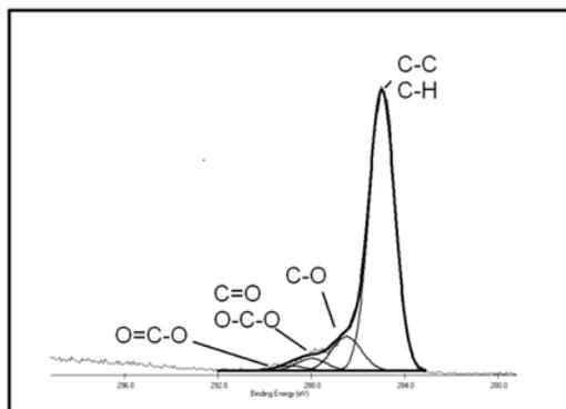
Figure 3. C1s measured for acetone plasma treated graphite surface for 20min.
