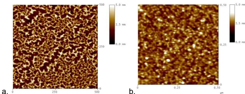
Figure 4. Topographic AFM images of HSA solution of concentration 0.001mg/ml adsorbed onto acetone plasma modified graphite surface: a. Overnight dried; b. few minutes dried
