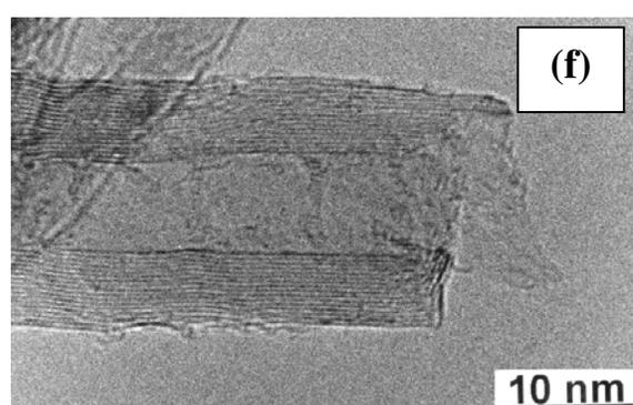
Figure 1. Electron microscopy images on the nanotubes NTNaY .
