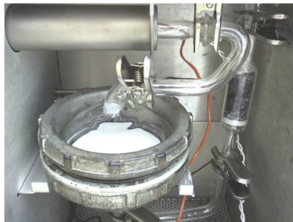
Figure 1. The interior of the hot box, with the adsorption reactor in operating position.
