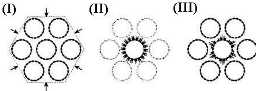
Fig. 1: Three scenarios by which the external pressure can be transmitted to bundled SWNTs (see ...)
