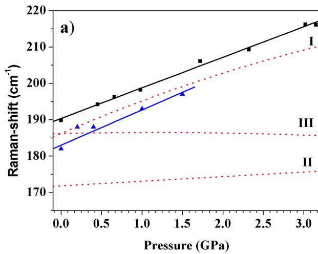
Fig. 3a : Experimentally determined pressure dependence for  $\omega_R$  in S-SWNTs (squares) and bundled tubes (triangles). The solid lines represent linear fits to the data. The dashed lines are theoretical pressure dependence of  $\omega_R$  in Models I – III (see text).
