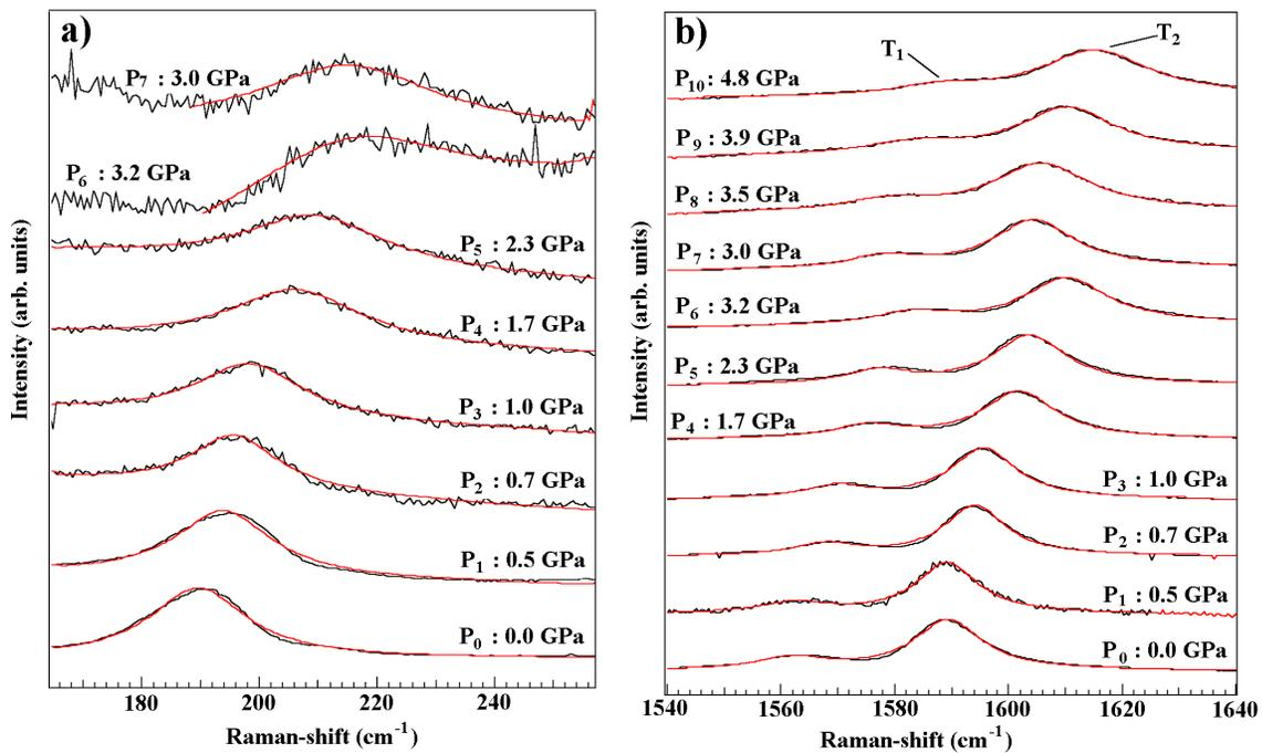
Fig. 2: Raman spectra of the radial (a) and tangential bands (b) that were observed for S-SWNTs at the indicated pressures.
