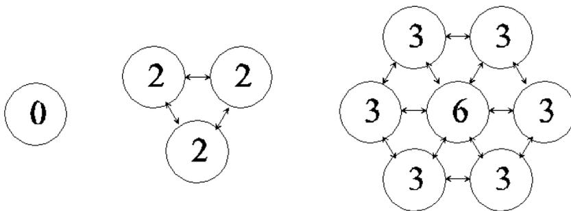
Fig. 4 : Schematic representation of small bundles found in S-SWNT samples used in this study. The numbers inside the circles represent the number of neighbors within the bundle.
