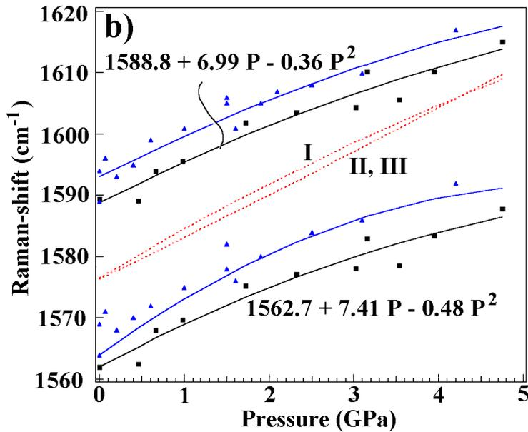
Fig. 3b : Quadratic fits (solid curves) for the two tangential mode frequencies observed in S-SWNTs (squares) and bundled tubes (triangles). The dashed lines represent model calculations discussed in Ref. 1.
