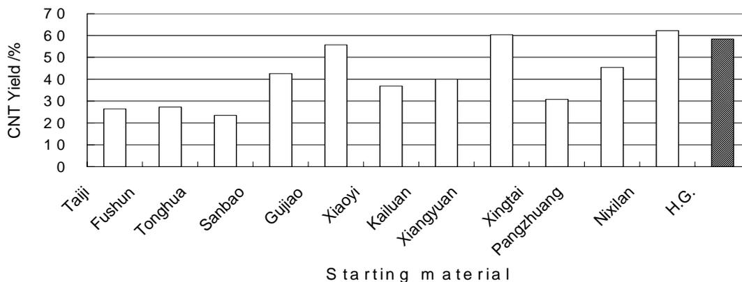
Figure 2 Yield of carbon nanotubes from different coals
