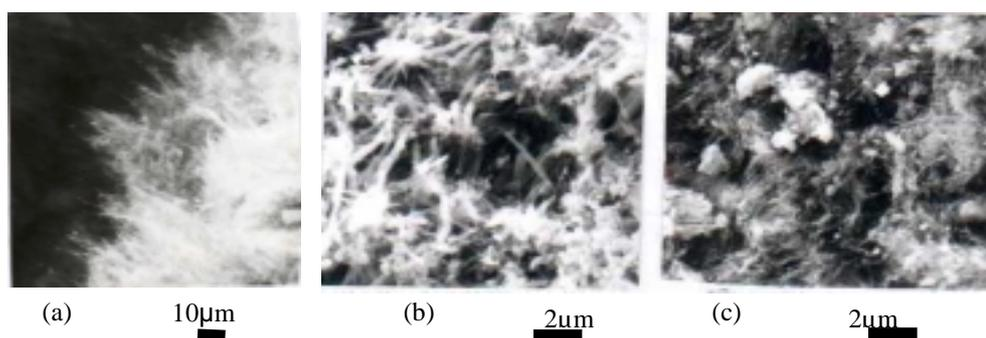
Figure 1. SEM photographs of carbon nanotubes from Xiangyuan coal and New Zealand coal (a) Xiangyuan coal, 0.03MPa; (b) Xiangyuan coal, 0.0665MPa; (c) New Zealand Coal, 0.03MPa
