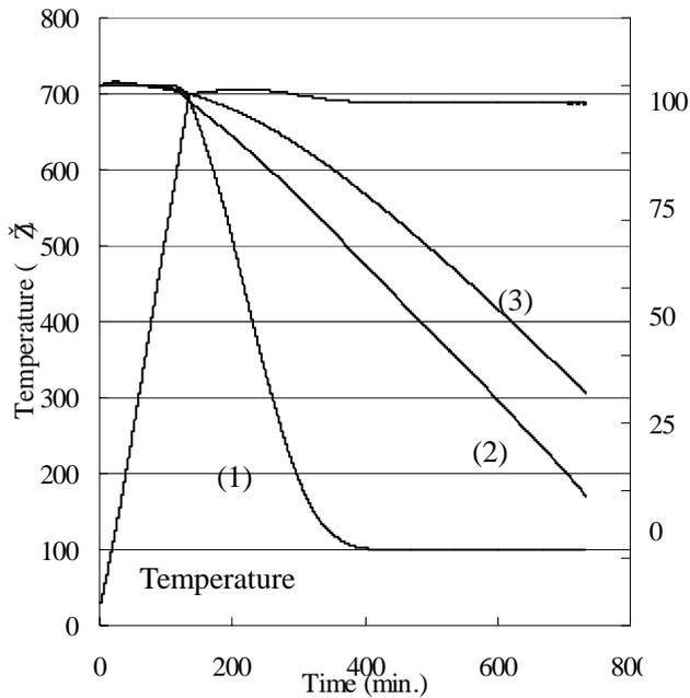
Fig.1 Non-Catalytic Isothermal Combustion of 3 kinds of Graphite Materials in  $N_2/O_2=7/3$  at 700
