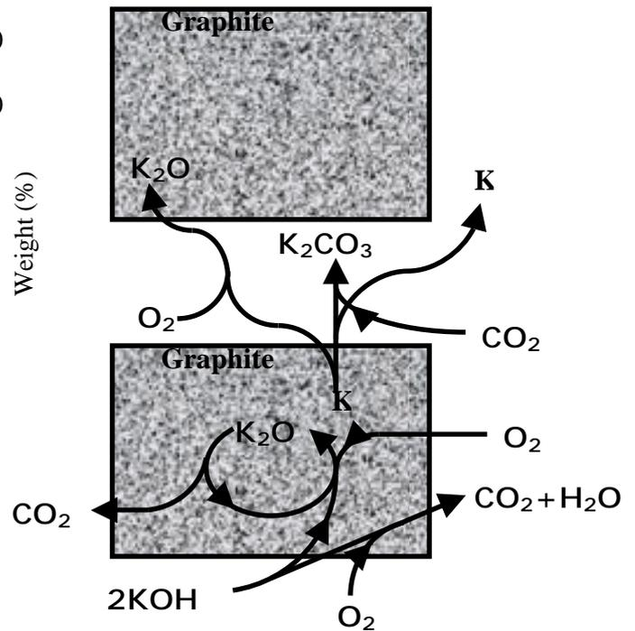
Fig.4 The Mechanism of the Catalytic Combustion of Graphite
