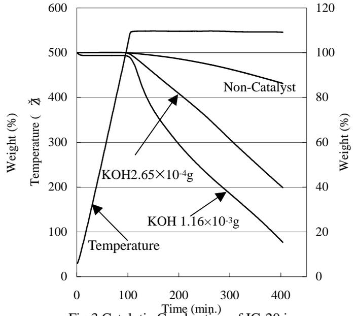
Fig.3 Catalytic Combustion of IG-20 in  $N_2/O_2=1$  at 550
