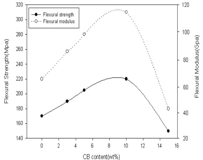
Fig.3. Flexural strength and modulus of C/C plate with different CB content
