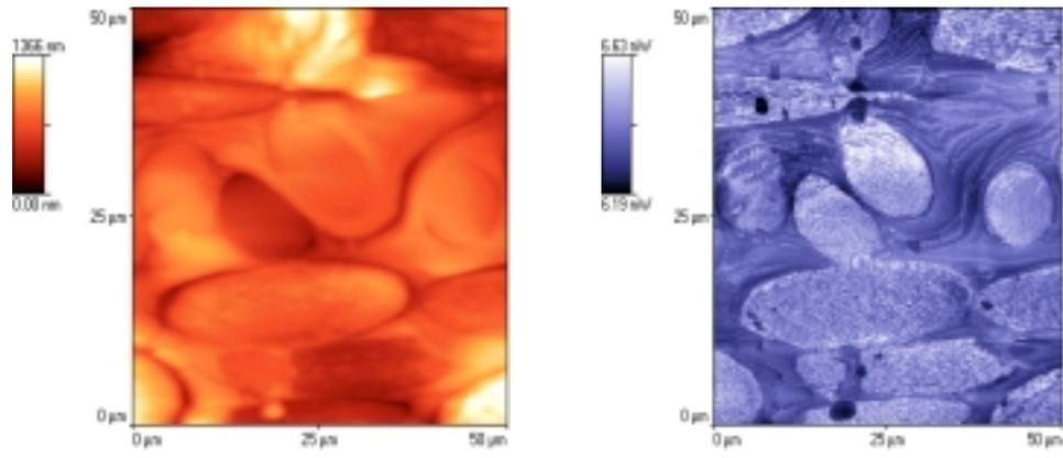
Fig.2 Topographical and Thermal image of F4M3 sample heat treated to 1000 C
