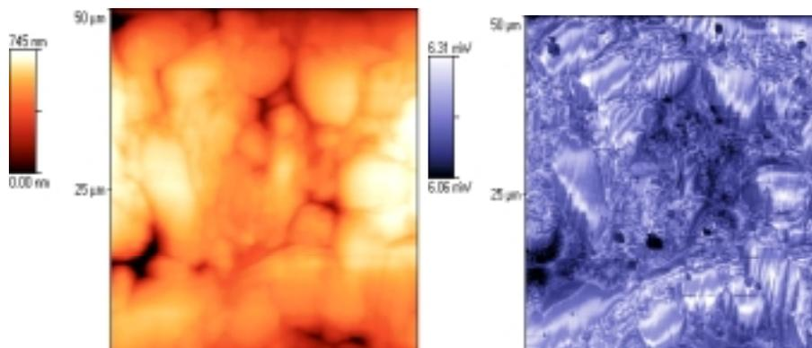
Fig.3 Topographical and Thermal image of F1M1 sample heat treated to 1000 C
