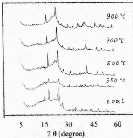
Figure 1 X-ray diffraction profiles of middle rank coal carbonized at various temperature
