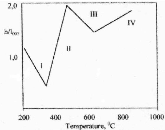
Figure 2 Alteration  $h/l_{002}$  parameter from carbonization temperature
