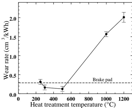
Figure 3. Wear rate as a function of HTT.
