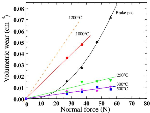
Figure 2. Volumetric wear as a function of the normal force applied.
