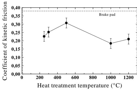
Figure 1. Coefficient of kinetic friction as a function of HTT.
