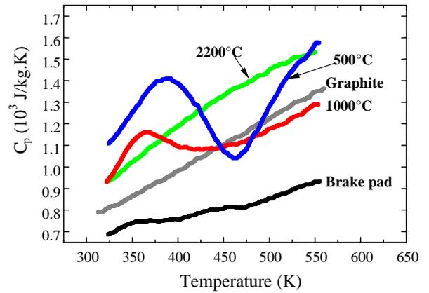
Figure 5. Specific heat as a function of temperature. The sample of 2200°C and the graphite are shown only for comparison.
