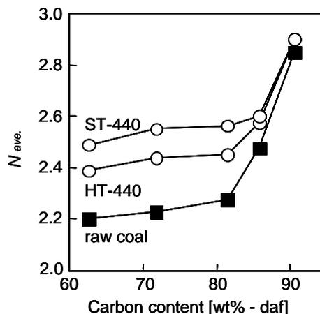
Figure 3. Change of  $N_{ave}$  for coals heat- or solvent-treated at 440°C.
