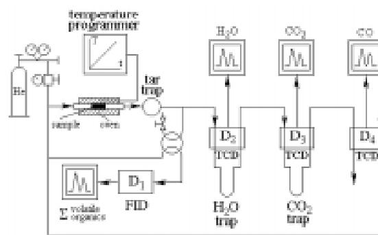
**Figure 1.** Schematic diagram of the setup for continuous analysis of cellulose pyrolysis gaseous products: TCD – thermal conductivity detector; FID – flame ionization detector.
