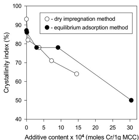
**Figure 4.** Variations in crystallinity indices of (NH<sub>4</sub>)<sub>2</sub>Cr<sub>2</sub>O<sub>7</sub>-doped MCCs with chromium content.
