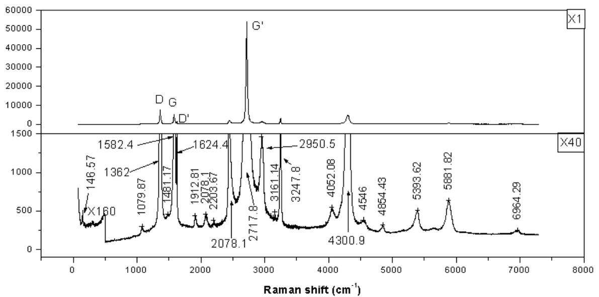
Fig 5 Raman spectra of carbon whisker with 488 nm excitation
