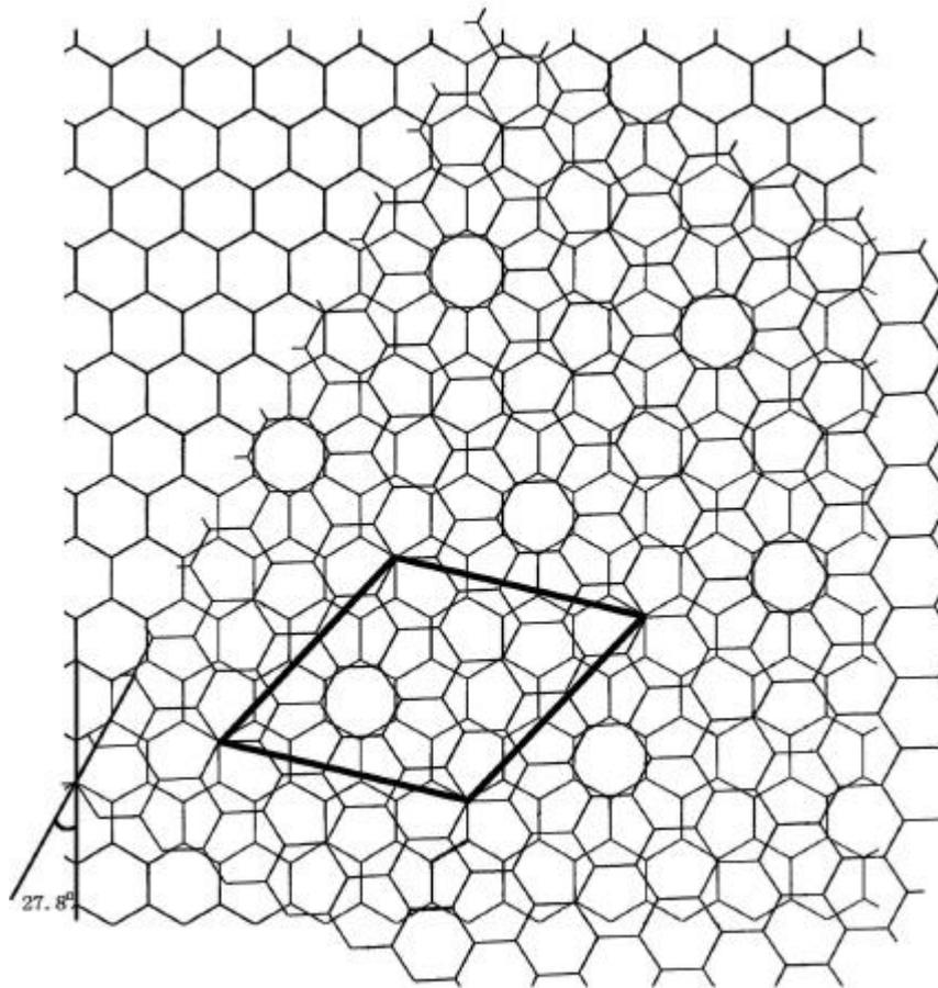
Fig 4 Schematic diagram of stack sequence of carbon layers in term of dclination
