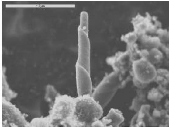
Fig 1 SEM micrograph of carbon whisker
