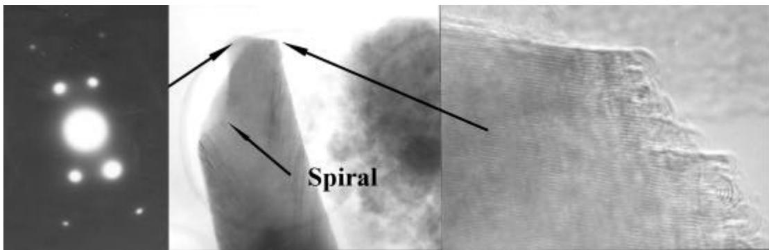
Fig 2 TEM micrograph of carbon whisker
