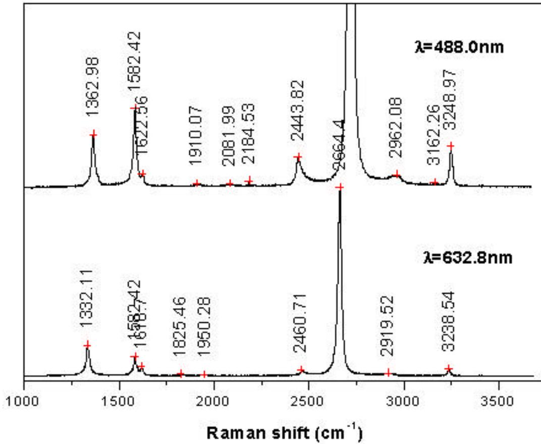
Fig 6 Raman spectra of carbon whisker with 488 and 632.8 nm excitation
