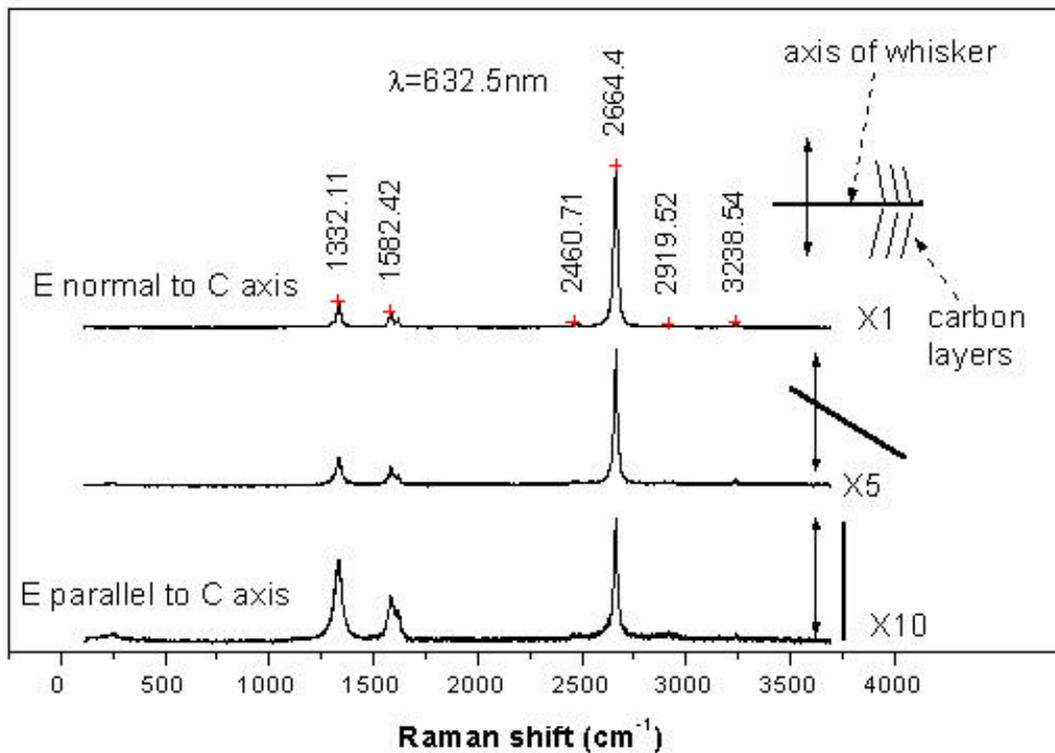
Fig 7. Polarized Raman spectra of carbon whiskers.
