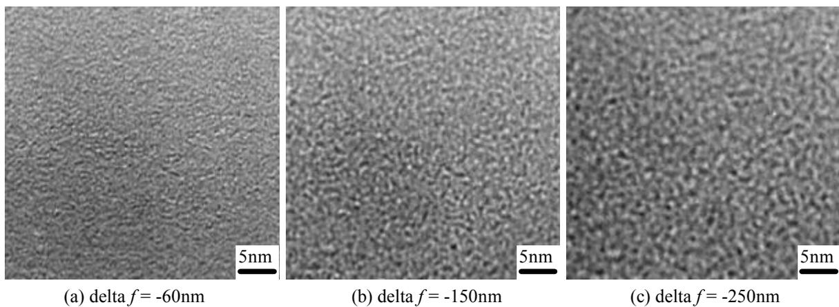
Figure 2. The TEM images for different  $\Delta f$ 's of JEM4000EX.
