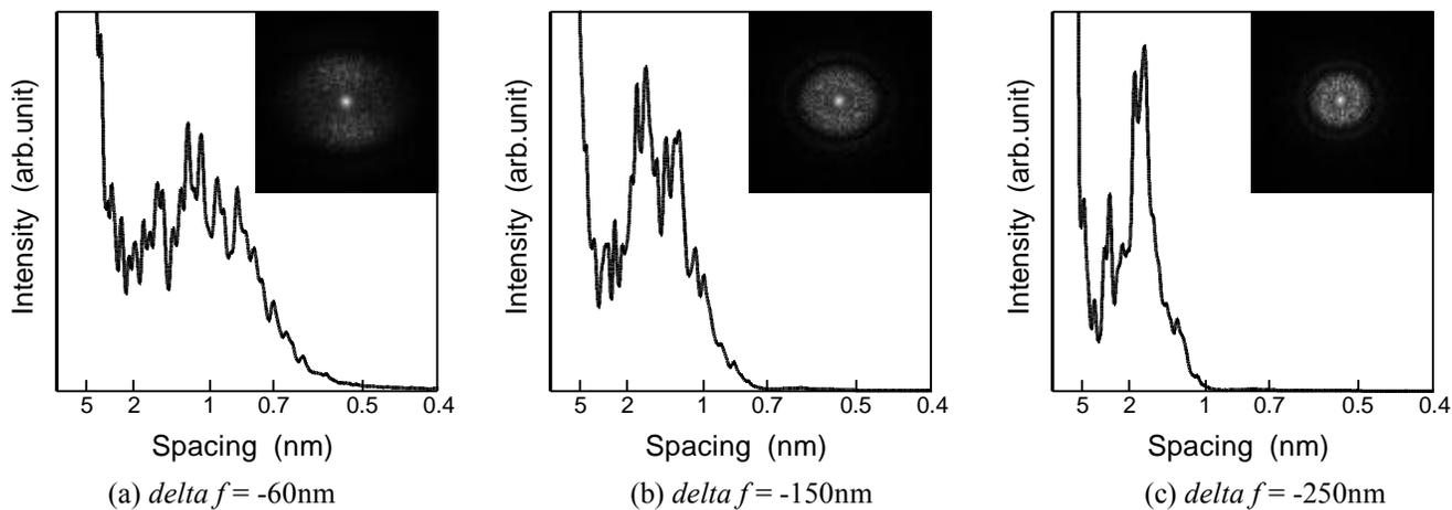
Figure 3. The insets power spectra for different  $\Delta f$ 's of JEM4000EX are integrated around the center points of them.
