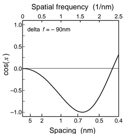
Figure 4. The phase transfer function for  $\Delta f = -90\text{nm}$  of JEM2010FEF. The value of  $\Delta f$  approximately corresponds to that of JEM4000EX at  $\Delta f = -90\text{nm}$ .
