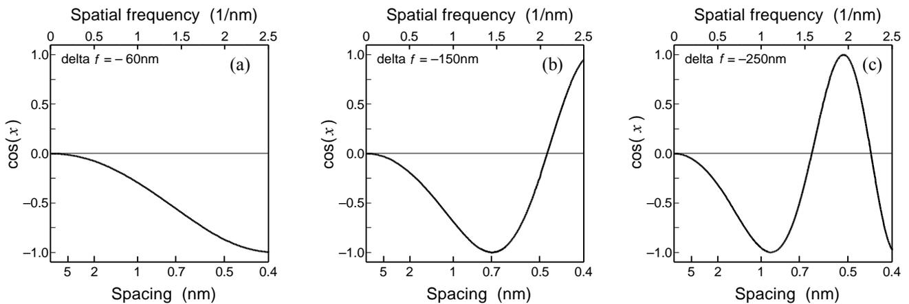
Figure 1. The phase transfer functions for different  $\Delta f$ 's of JEM4000EX.
