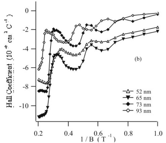
Fig.2. Hall coefficient  $R_H$  of graphite films of various thickness as a function of the reciprocal of the magnetic field  $B$  at 1.8K, (a) films thinner than about 50 nm, (b) films thicker than about 50 nm.
