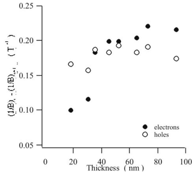
Fig.3. Film thickness dependence of the period of Shubnikov - de Haas oscillation.
